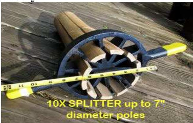
Fig10: Bamboo Splitting
