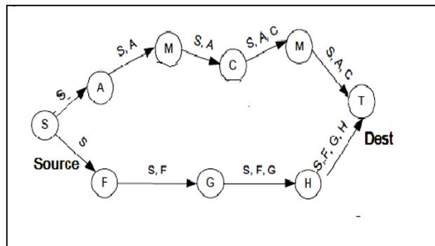
Figure 1. Example for SRP routing.
