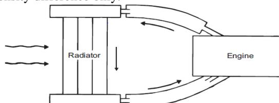
Figure 5.2 : Thermo Siphon System of Cooling
