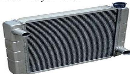
In automobiles and motorcycles with a liquid cooled internal combustion engine, a radiator is connected to channels running through the engine and cylinder head, through which a liquid (coolant) is pumped. This liquid may be water (in climates where water is unlikely to freeze), but is more commonly a mixture of water and antifreeze in proportions appropriate to the climate.
