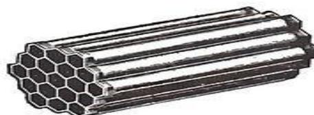
Internal combustion engines are often cooled by passing a liquid called *engine coolant* through the engine block, where it is heated, then through the radiator itself where it loses heat to the atmosphere, and then back to the engine in a closed loop. Engine coolant is usually water-based, but may also be oil. It is common to employ a water pump to force the engine coolant to circulate, and also for an axial fan to force air through the radiator.
