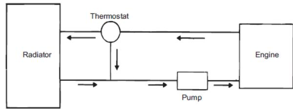
Figure 5.4 : Water Cooling System using Thermostat Valve
