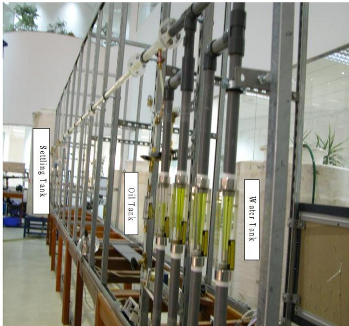
Figure 1 Photograph of the flow loop
