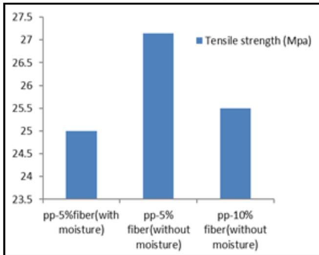
Fig 1: The tensile strength of the composites
