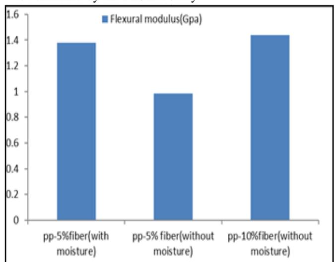
Fig 4: The flexural modulus of the composites
