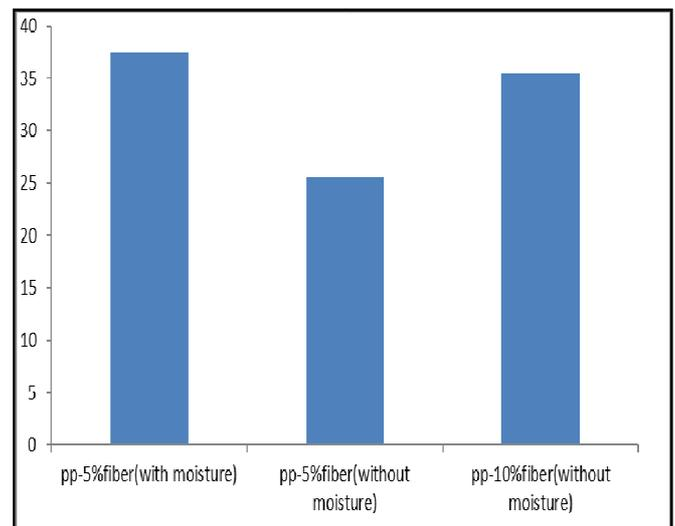
Fig 3: The flexural strength (MPa) of the composites
