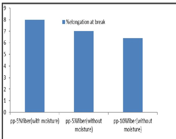
Fig 2: The % elongation at break of the composites
