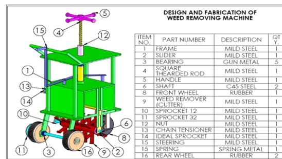
**Fig 1 design of weedremoving machine**
