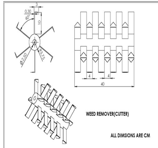
Fig 7 Dimensions of weed remover (cutter)
