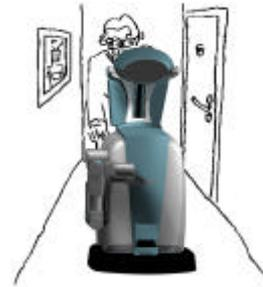
Fig. 2. Care-O-bot being used as an intelligent walking aid.
