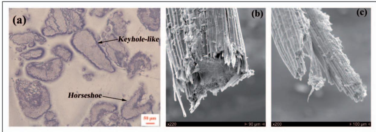
**Figure 1.** (a) Optical micrograph showing the cross-section of several *P. tenax* fibers; (b, c) SEM micrographs of *P. tenax* fibers fractured in tension.
