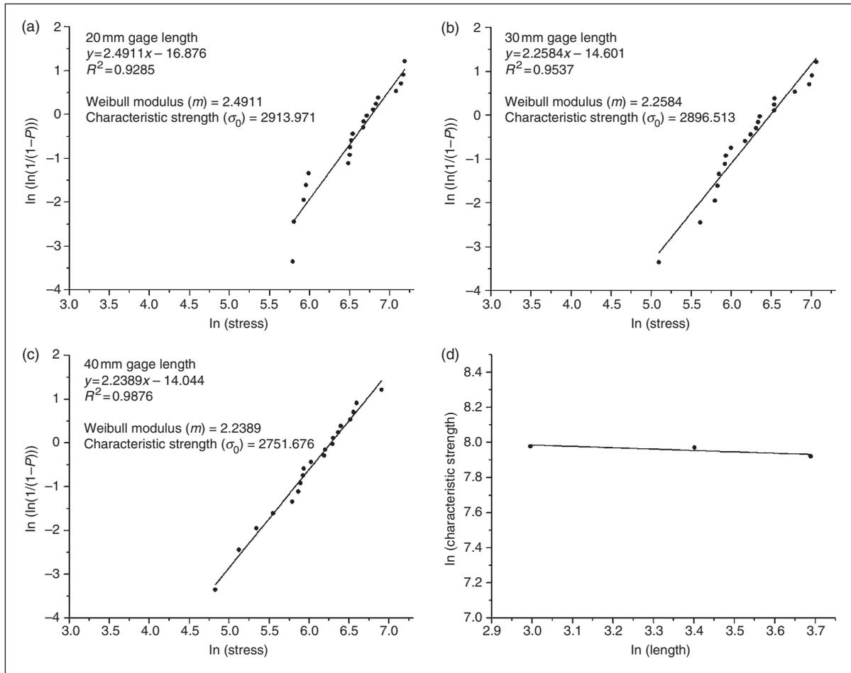
**Figure 3.** Weibull plots for *P. tenax* fibers tested at (a) 20 mm; (b) 30 mm; and (c) 40 mm; (d) weak link scaling plot.
