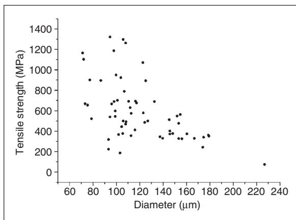
**Figure 2.** Tensile strength as a function of *P. tenax* fiber diameter.
