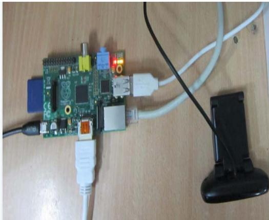
Fig 2: Connection Of USB Camera With Raspberry Pi
