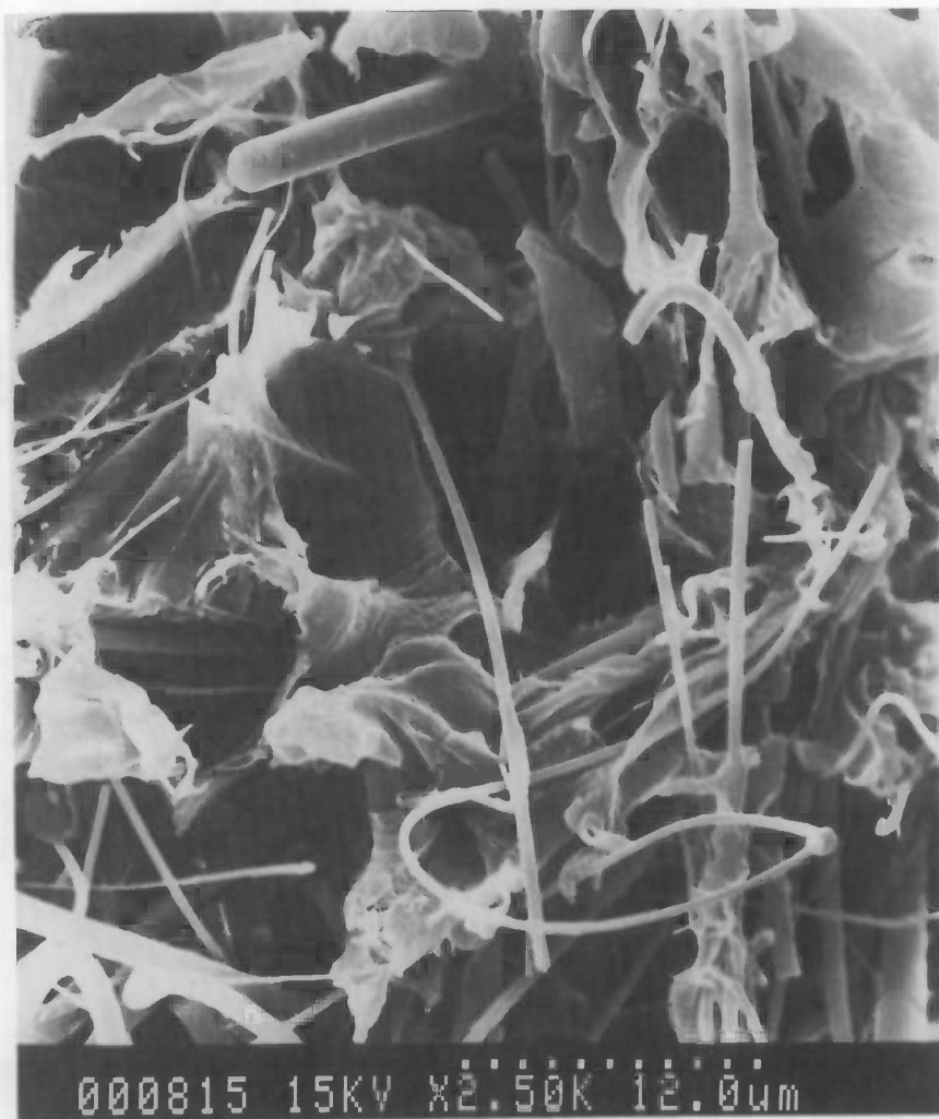
Figure 2. A torn section of the glass filter paper sandwiched between the plastic scintillator (broken granules of wrinkled and cracked plastic scintillator are folded among the glass fibers).
