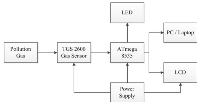
Fig. 1. Basic diagram of monitoring air pollution system.
