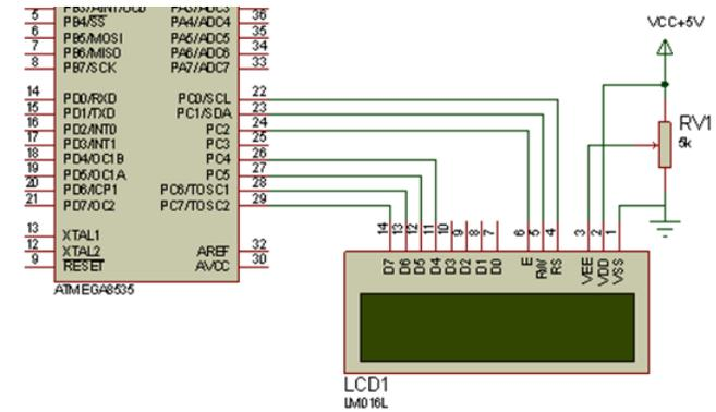
Fig. 6. The LCD circuit connection to the microcontroller
