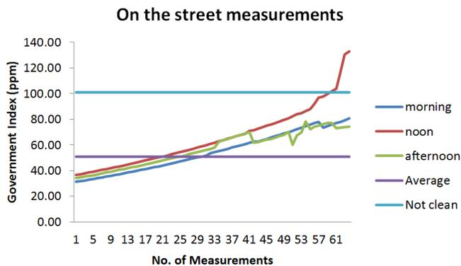
Fig. 16. Index measurement on the street path during morning, noon and afternoon
