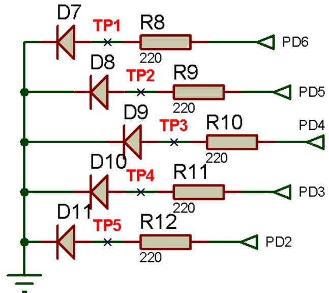
Fig. 13. Location of Indicator circuit measurements
