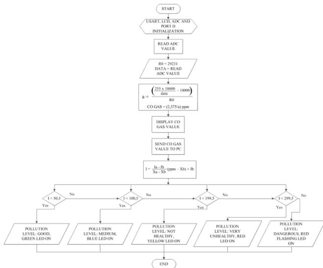
Fig. 8. Flowchart of software design of air pollution monitoring system
