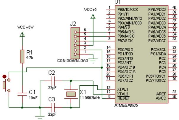
Fig. 5. Microcontroller circuit of ATMEGA8535
