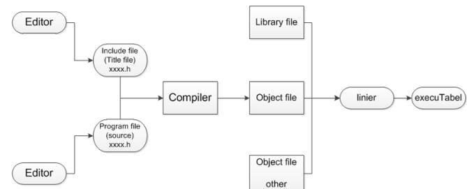
Fig. 12. Schematic of the hex file development in C compiler
