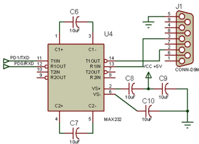
Fig. 7. Serial interface circuit of IC MAX232
