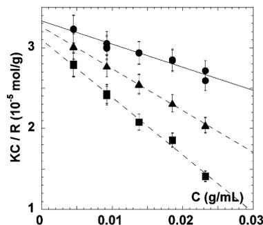
**Figure 2.**  $KC/R$  as a function of the polymer concentration  $C$  for PDMS samples with  $M_w = 31$  kDa at a  $\text{CO}_2$  density of 0.97 g/mL and three different temperatures: (■) 25, (▲) 37, and (●) 54 °C.
