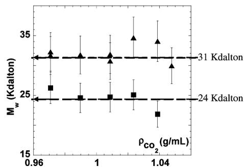
**Figure 3.** Molecular weights determined by light scattering in  $\text{CO}_2$  at 25 °C, plotted as a function of the  $\text{CO}_2$  density for two samples: (■) 24 and (▲) 31 kDa. Dashed lines at 24 and 31 kDa correspond to the molecular-weight values measured in benzene.
