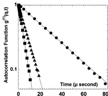
**Figure 1.** Semilogarithmic plot of the field autocorrelation functions ( $g^{(1)}(q,t)$ ) obtained at 25 °C for PDMS samples with a molecular weight of  $M_w = 31$  kDa, a  $\text{CO}_2$  density of 1.04 g/mL, and a polymer concentration of  $C = 0.0232$  g/mL. Different sets of symbols correspond to wavevectors: (■) 0.0284, (▲) 0.0216, and (●) 0.0107  $\text{nm}^{-1}$ .
