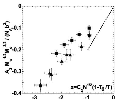
**Figure 7.** Reduced second virial coefficient of PDMS samples with molecular weights of (■) 24 and (▲) 31 kDa in CO<sub>2</sub> at a density of 0.97 g/mL. Linear extrapolation of the universal curve into the negative A<sub>2</sub> regime is represented by the dashed line.
