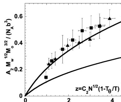
**Figure 6.** Normalized second virial coefficient plotted as a function of the interaction parameter for PDMS samples with molecular weights of (■) 24 and (▲) 31 kDa in benzene. The data previously obtained in traditional organic solvents (not shown) are located between the two solid curves.<sup>9,37–39</sup>
