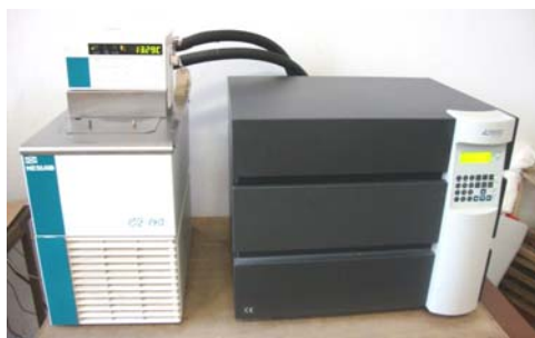
Fig. 3 Apparatus Holometrix 2300 for determination of thermal conductivity
