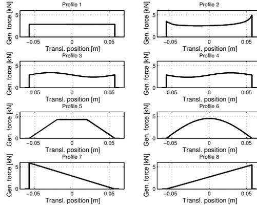
Figure 2: Generator force as a function of translator position when the translator is moving from left to right.
