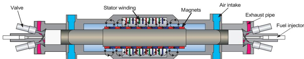
Figure 1: A Free Piston Energy Converter
