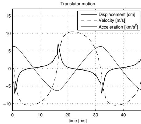
Figure 4: Typical free piston displacement, velocity and acceleration from simulation.
