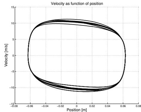
Figure 6: Translator velocity as a function of position.
