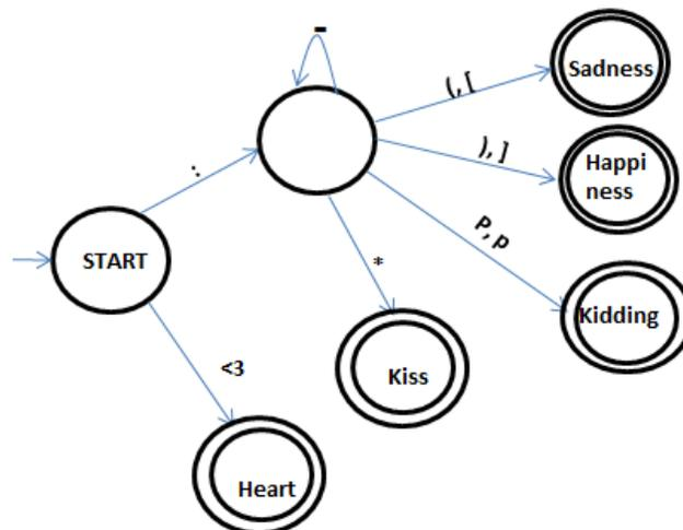
Figure 1: Finite State Machine which exploits Emoticons to determine text polarity.
