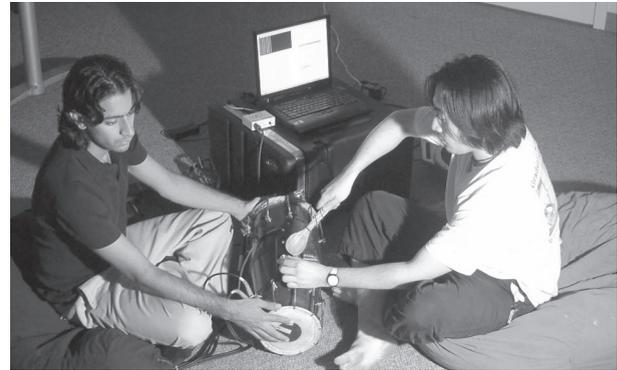
Figure 4. EDholak: a two-person electronic drum.
