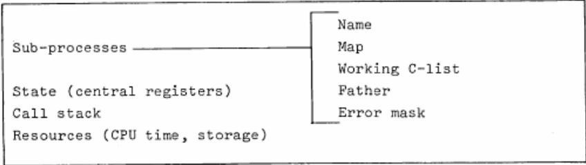
**Figure 3:** Components of a process
