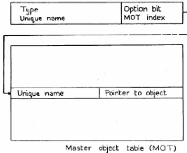
**Figure 4:** The structure of a capability
