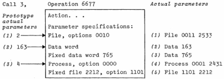
**Figure 5:** Calling an operation: constructing the actual parameter list
