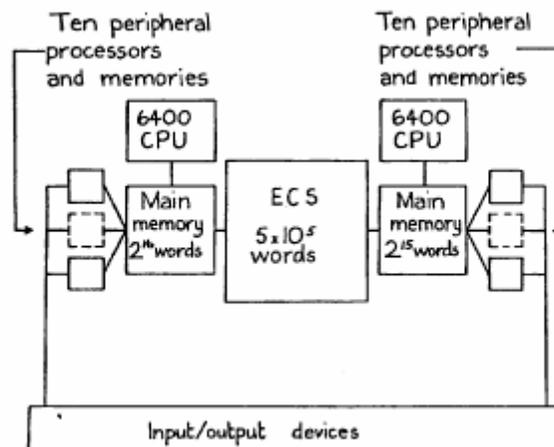
**Figure 1:** Dual 6400 hardware configuration
