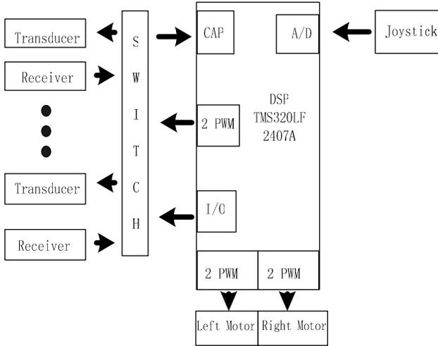
Fig. 2 Hardware configuration
