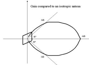
Fig. 5. Radiation pattern schematic for a patch antenna [9]
