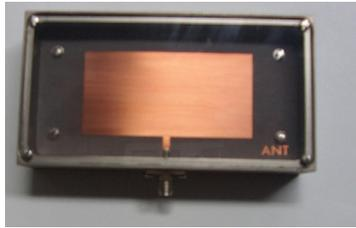
Fig. 4. Micro-strip patch antenna for 1-3 GHz [9]
