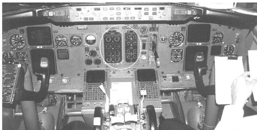
Figure 1: A 737-400 cockpit. The EIS is located in the centre (see white circle). © Pedro Becken.
