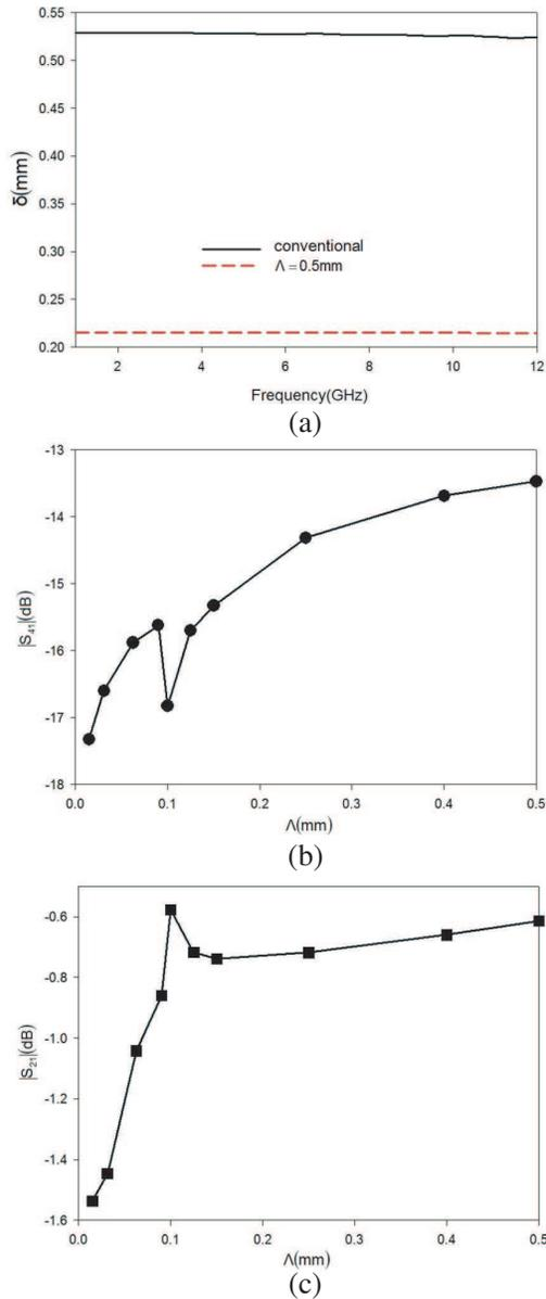
**Figure 3.** (a) Field decay length as a function of frequency. (b) Dependence of  $S_{41}$  on period  $\Lambda$ . (c) Dependence of  $S_{21}$  on  $\Lambda$ . The length of the coupled strip lines are  $L = 5$  cm.
