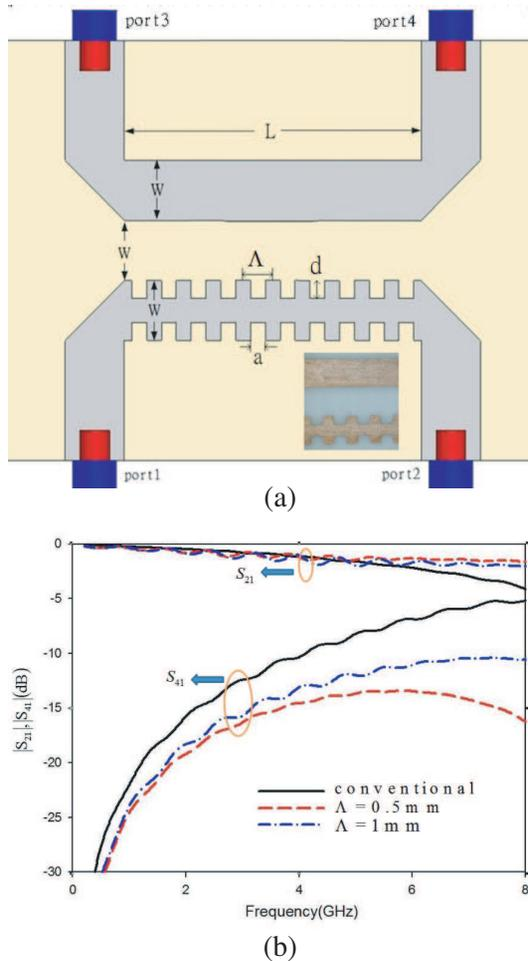
**Figure 4.** (a) Experimentally measured structure: Periodically corrugated couple metal strip line, (b) experimentally measured data of  $S$  parameters with the groove depth  $d = 0.3w$  and  $\bar{a} = a/\Lambda = 0.5$ .
