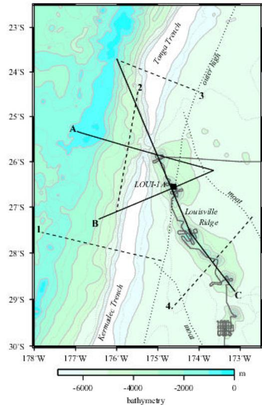
**Fig. 5:** Acquisition geometry showing the location of *Profiles A-C* (solid black lines) relative to the Louisville Ridge and Tonga-Kermadec Trench. Square – IODP drill site LOUI-1A. Existing R/V Sonne *Profiles 1-4* are shown by dashed lines. Thin grey lines show existing swath bathymetry tracks [*Koppers et al., 2004*].
