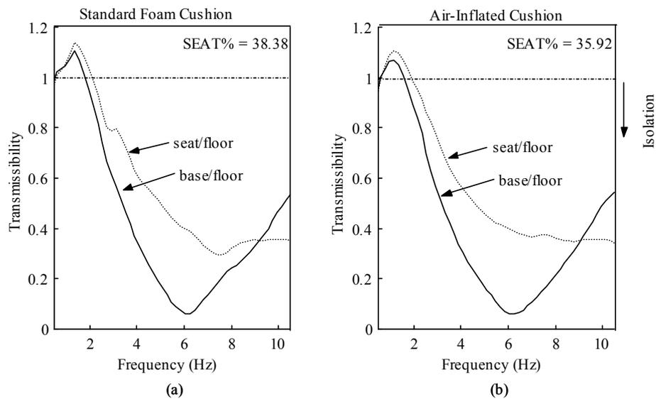
Figure 12 Vertical transmissibility (base acceleration divided by floor acceleration and seat acceleration divided by floor acceleration); (a) standard foam cushion; (b) air-inflated cushion.
