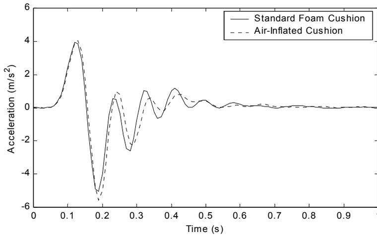
Figure 10 Vertical seat acceleration response to a 1-inch step input.
