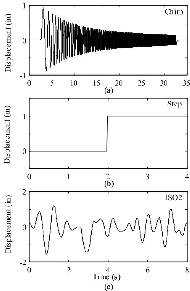
**Figure 6** Time traces of experimental input signals: (a) Chirp; (b) Step; (c) ISO2.
