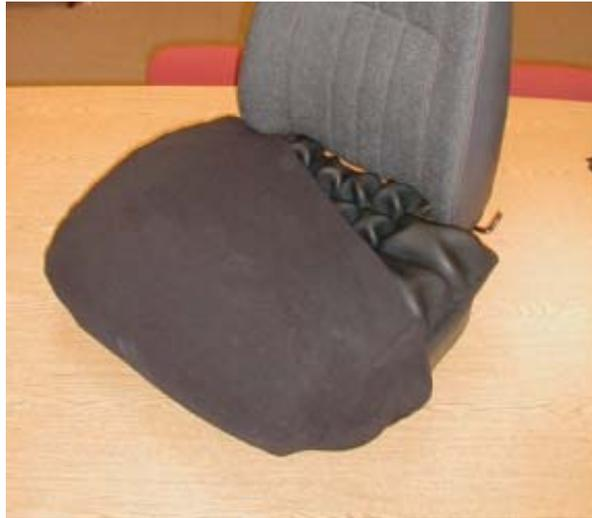
**Figure 2** *Experimental air-inflated seat cushion partially covered.*
