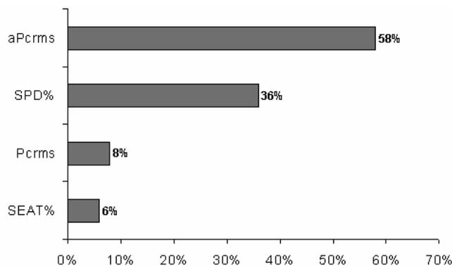
**Figure 21** Percent improvement offered by an air-inflated seat cushion in comparison with a foam cushion, using different metrics.
