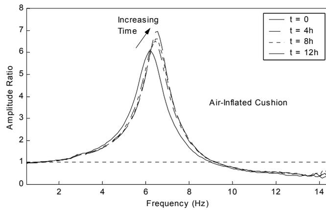
**Figure 8** Vertical cushion transmissibility (seat acceleration divided by base acceleration) for the air-inflated seat cushion.
