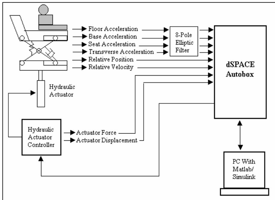
Figure 4 Data acquisition setup.
