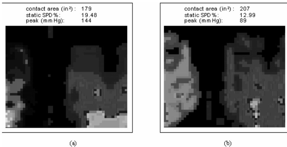
**Figure 13** Static interface pressure distribution; (a) standard foam cushion; (b) air-inflated cushion.
