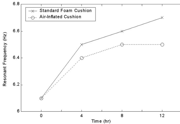
Figure 9 Change in resonant frequency over time.
