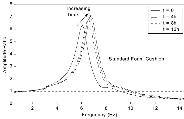
**Figure 7** Vertical cushion transmissibility (seat acceleration divided by base acceleration) for the standard foam cushion.
