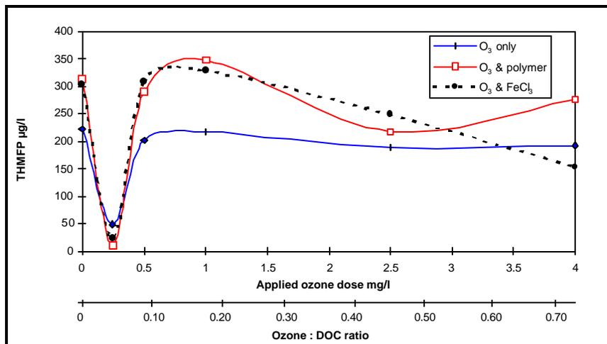
Figure 2: Effect of Pre-ozonation and conventional treatment on the THMFP of a eutrophic water (Inanda Dam water containing 100 000 *Microcystis* cells/ml).
