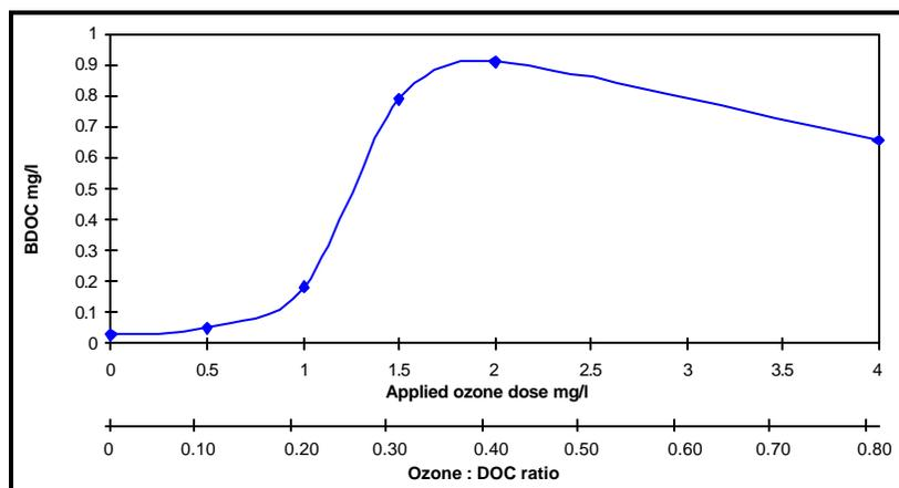
Figure 4 Effect of ozone on the BDOC of a final filtered water.
