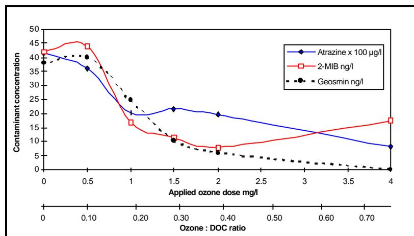
Figure 5: Effect of ozone on atrazine, geosmin and 2-MIB of a final filtered water.
