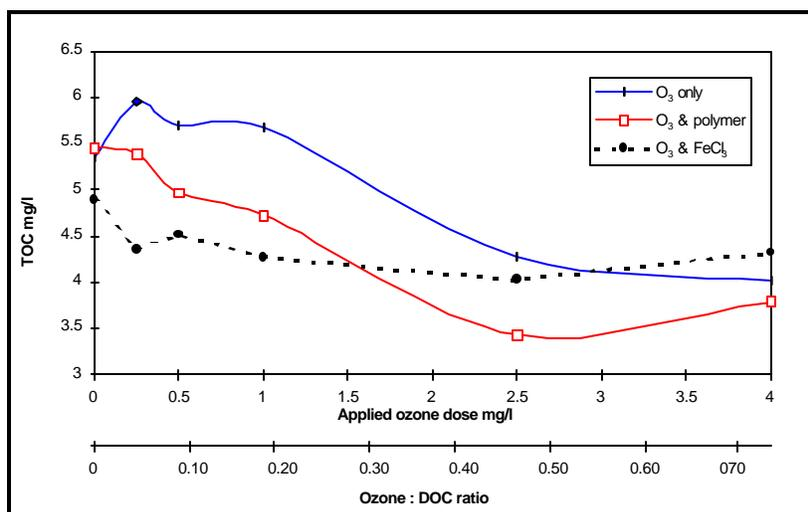
Figure 3 Effect of ozone on the TOC of an eutrophic water (Inanda Dam water containing 100 000 *Microcystis* cells/ml).
