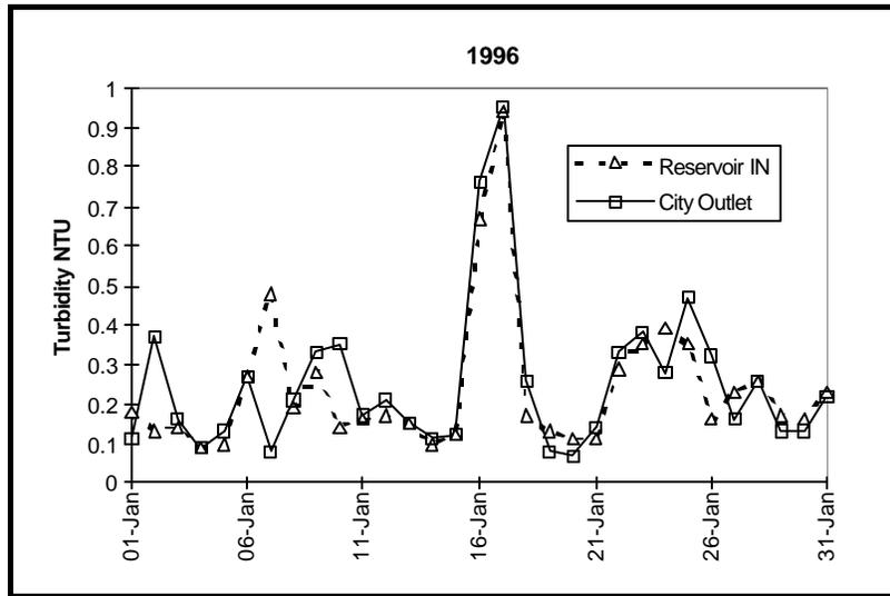
Figure 6: Turbidity entering and exiting the reservoir at Wiggins
