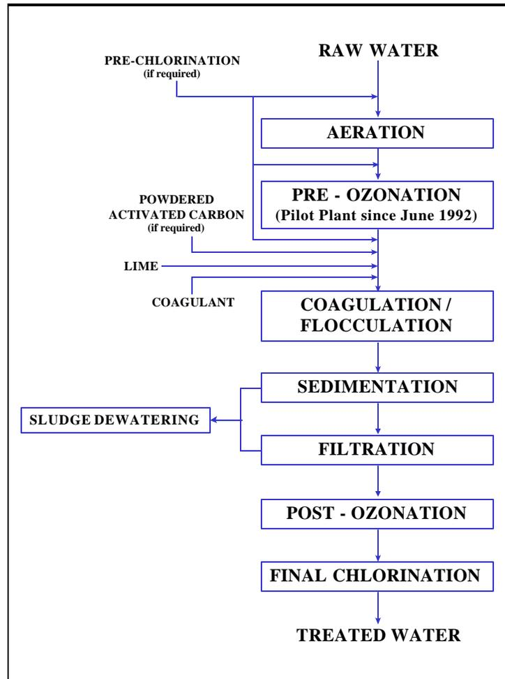
Figure 1 Schematic of Wiggins Waterworks treatment (prior to 1997)
