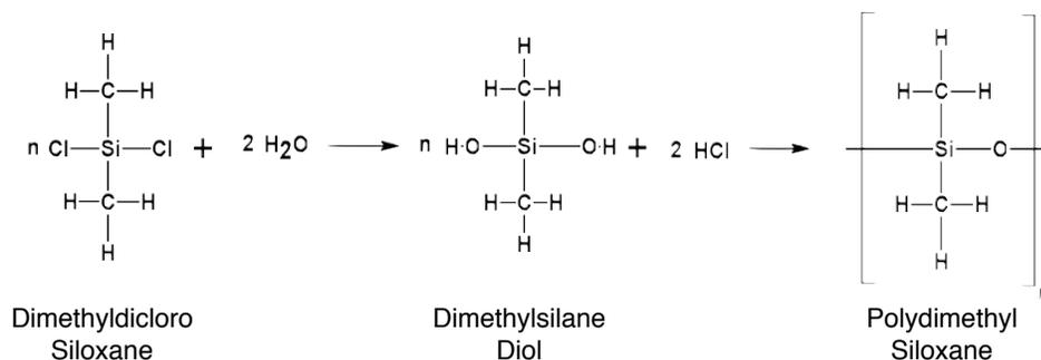
Figure 1: Polymerization of Dimethyl Siloxane
