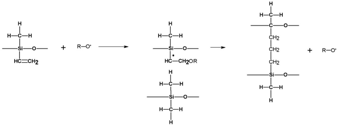
Proposed Crosslink Reaction for VMQ — crosslink is followed by termination step
