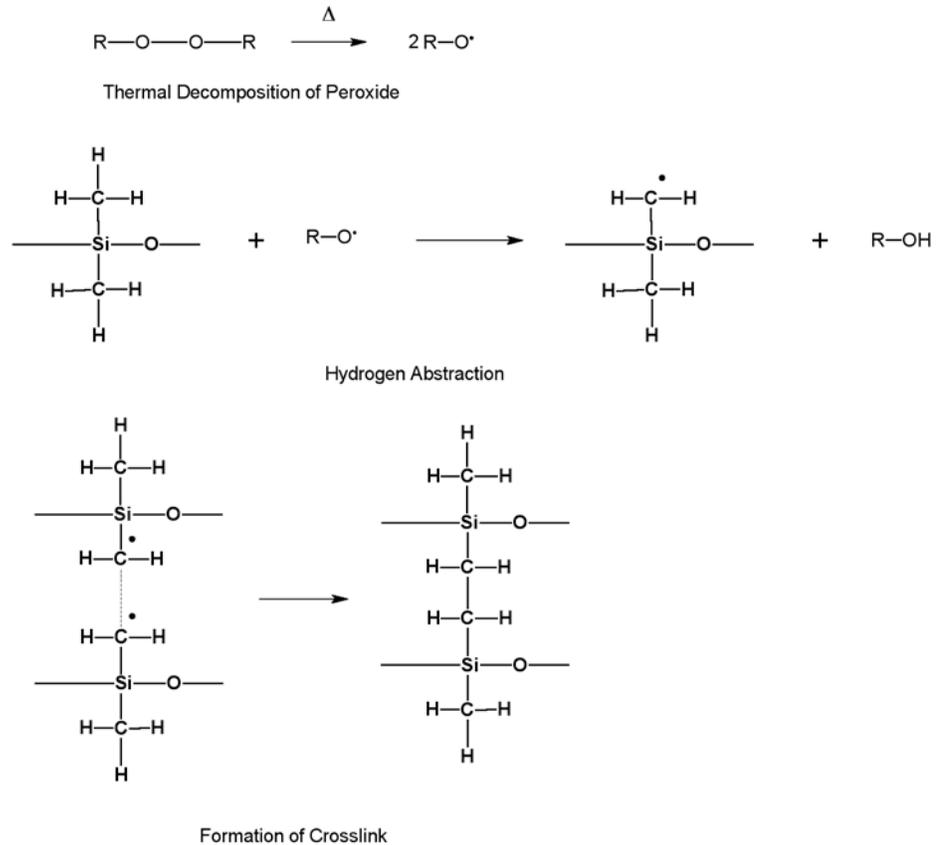
**Figure 3:** Three-step crosslink reaction for peroxide cure of MQ
