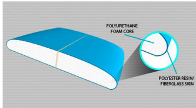
**Figure 2: Cutaway of conventional surfboard construction. Image from Stewart surfboards website (4).**
