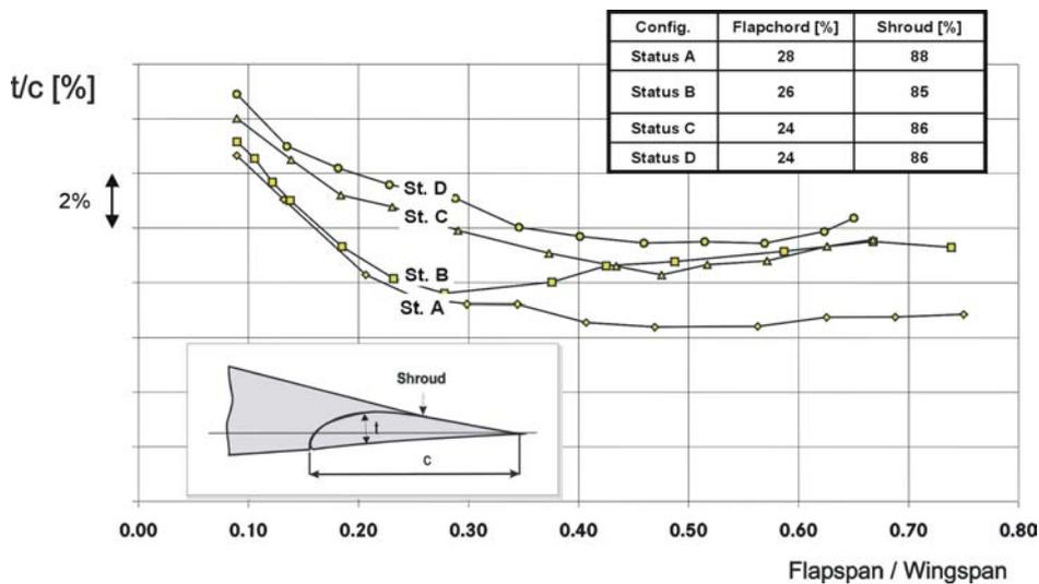
Figure 12: Evolution of the trailing edge device layout
