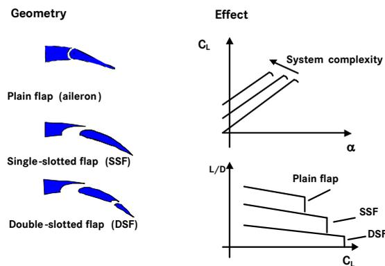
Figure 3: Trailing edge devices
