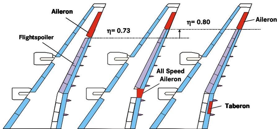
Figure 11: Variation of the trailing edge and roll control concept
