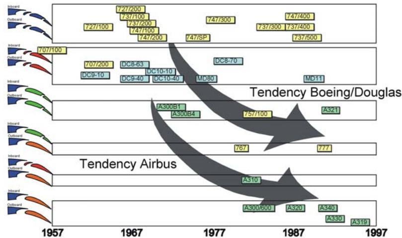
Figure 4: Design evolution of high-lift wing trailing edge systems [3]
