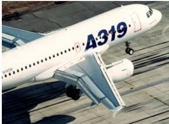
Figure 1: Airbus A319 wing in high-lift configuration
