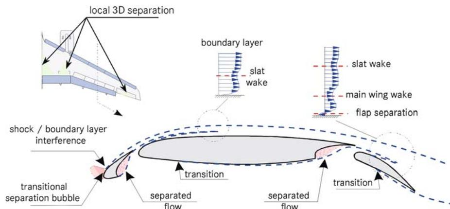
Figure 5: Flow phenomena on a high-lift wing
