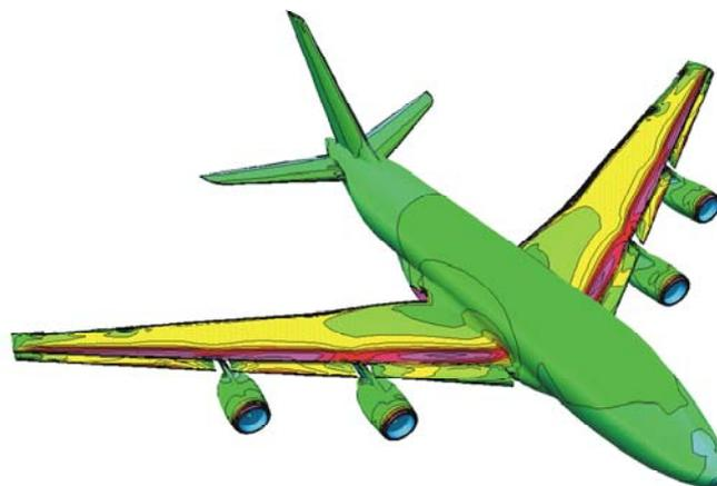
Figure 6: Flow analysis for the complete high-lift-configuration
