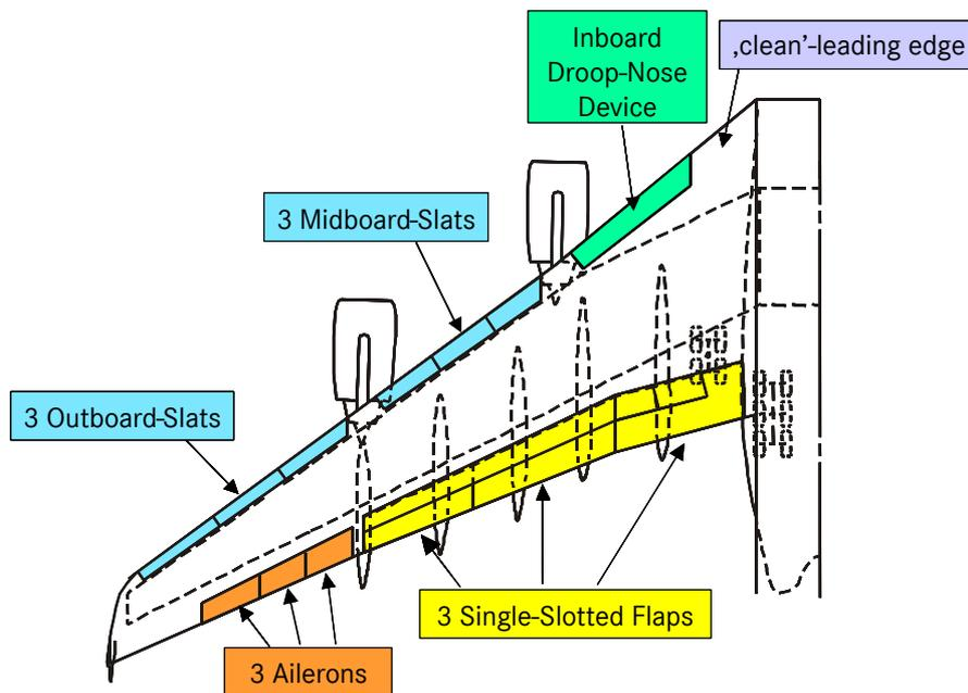
Figure 13: The Megaliner high-lift wing layout
