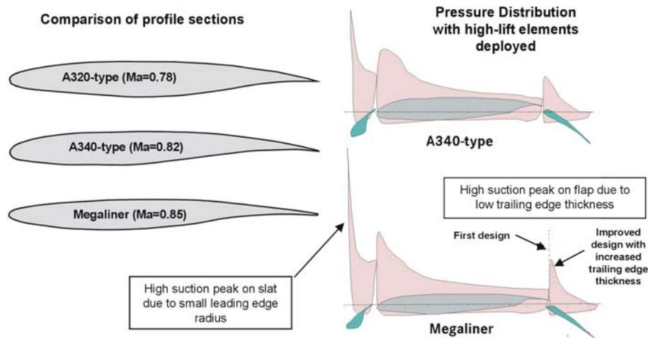
Figure 10: Comparison of Airbus profile sections and problem areas on the Megaliner high-lift wing profiles
