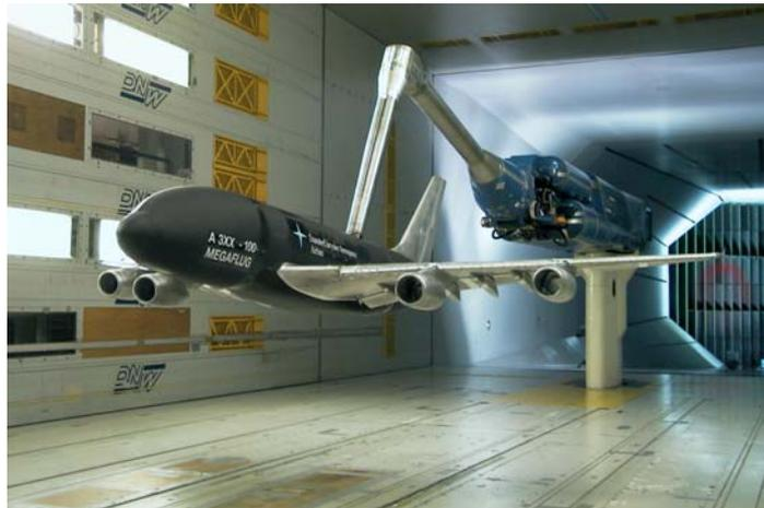
Figure 7: Megaliner complete-model in the DNW-LLF windtunnel
