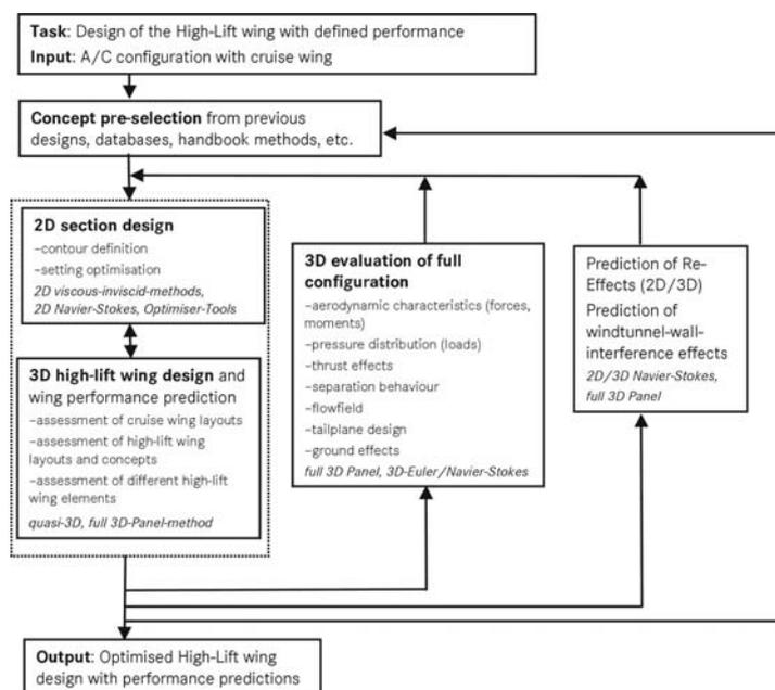
Figure 9: Sequence of the CFD-based high-lift design process
