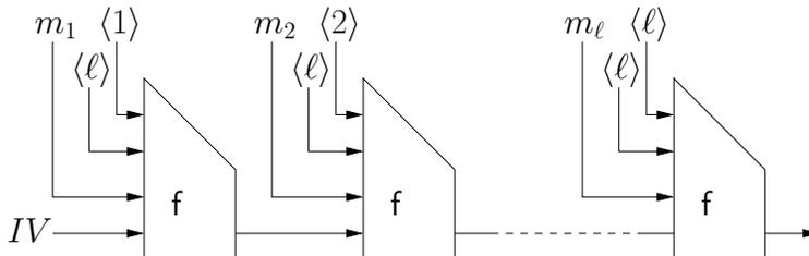
**Fig. 6.** Merkle-Damgård with a particular prefix-free encoding.
