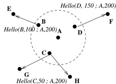
Figure 4: The information transmitted by node A is forwarded to nodes at two hops from A
