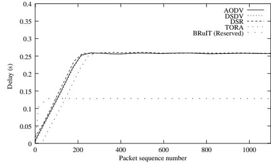
Figure 7: Filtering the flows has positive influence on delays when congestion appears
