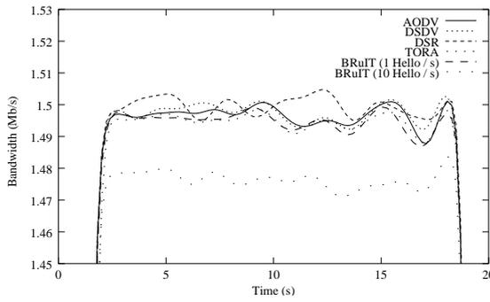
Figure 5: Maximum bandwidth between two nodes
