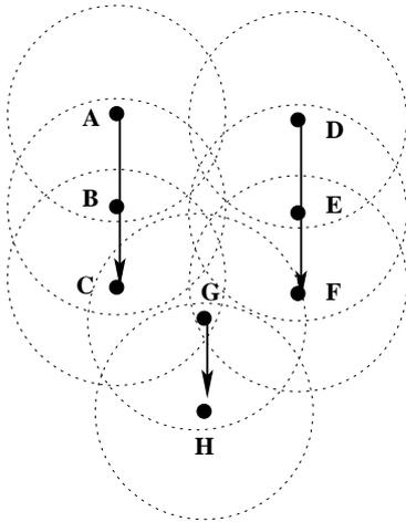
Figure 10: Three transmissions can interfere: *A* to *C* at 200 kb/s, *D* to *F* at 200 kb/s and *G* to *H* at 1Mb/s
