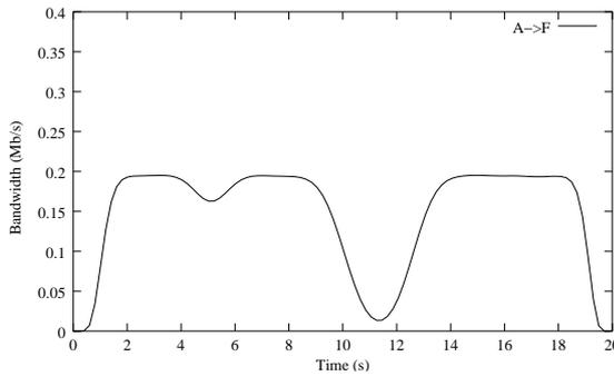
Figure 9: Time needed to rebuild a route broken due to mobility
