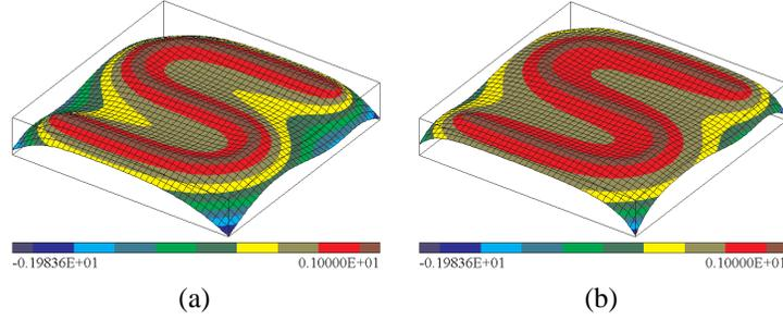
Figure 6: Approximation of the material function  $e^{(-1.5)u}$  shown in Figure 4(a) by the sum of generalized Taylor series terms shown in Figure 5: (a) First two terms  $1 + (-1.5)u$ . (b) First four terms  $1 + (-1.5)u + \frac{(-1.5)^2}{2!}u^2 + \frac{(-1.5)^3}{3!}u^3$ .
