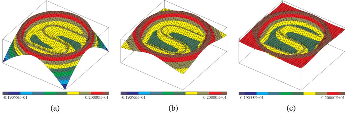
Figure 12: Inverse distance interpolation of two material functions with derivative control:  $P^1 = 1 - 1.5u$  is associated with the S-curve and  $P^2 = 2$  is associated with the circular ring. (a)  $k = 1$  for the S-curve and no derivative control; (b)  $k = 2$  means that the first derivatives on S-curve are interpolated exactly; (c)  $k = 3$  further decreases the influence of the S-curve feature
