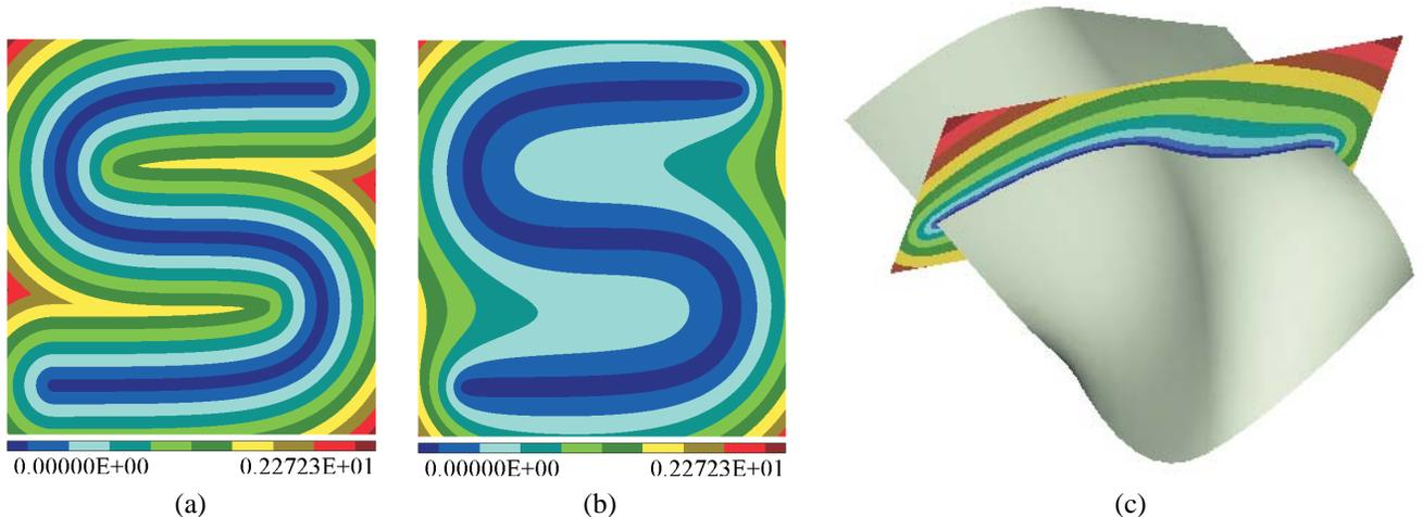
Figure 2: (a) The exact distance field of an S-shaped 4th-order B-spline curve; (b) An approximate distance field for the same curve normalized to the first order; (c) A section of an approximate distance field for a 4th-order B-spline surface normalized to the second order.
