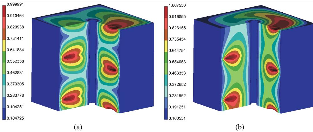
Figure 14: Transfinite interpolation of the material features in Figure 13: (a) Inverse distance interpolation. (b) Interpolation of (a) further constrained to satisfy the Laplace equation.
