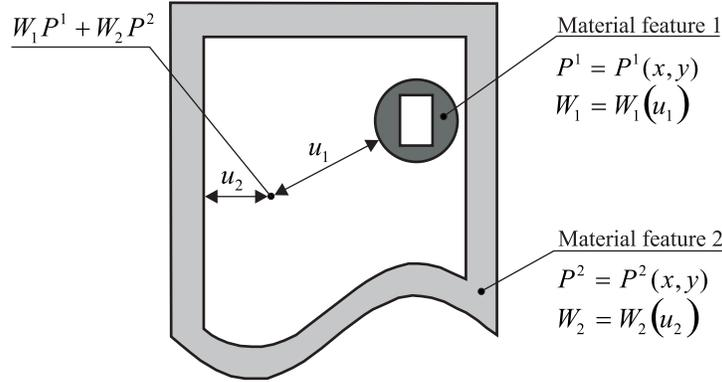
Figure 10: Example of material interpolation problem: construct a material function that combines material functions of individual features.
