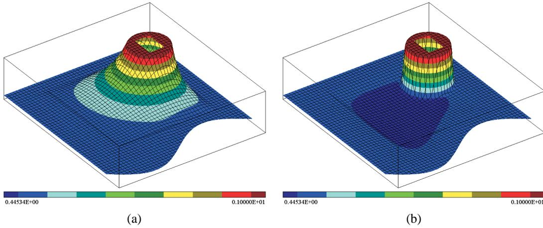
Figure 11: Transfinite interpolation of the material functions in Figure 10: specified material properties  $P^1 = 1$  and  $P^2 = 0.5e^{-u_2^2}$  are interpolated using first-order normalized distance fields. (a) Inverse distance interpolation; (b) weighted inverse distance interpolation with influence functions with  $\lambda_1 = e^{60u_1}$  and  $\lambda_2 = 1$ .
