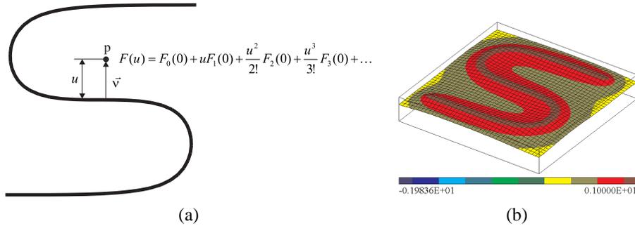
Figure 4: (a) A material function  $F$  may be represented in the neighborhood of the material feature, in this case S-curve, by a Taylor's series expansion in the powers of a distance field  $u$ . (b) Material function  $e^{-1.5u}$  is prescribed in terms of distance  $u$  to the S-shaped feature.
