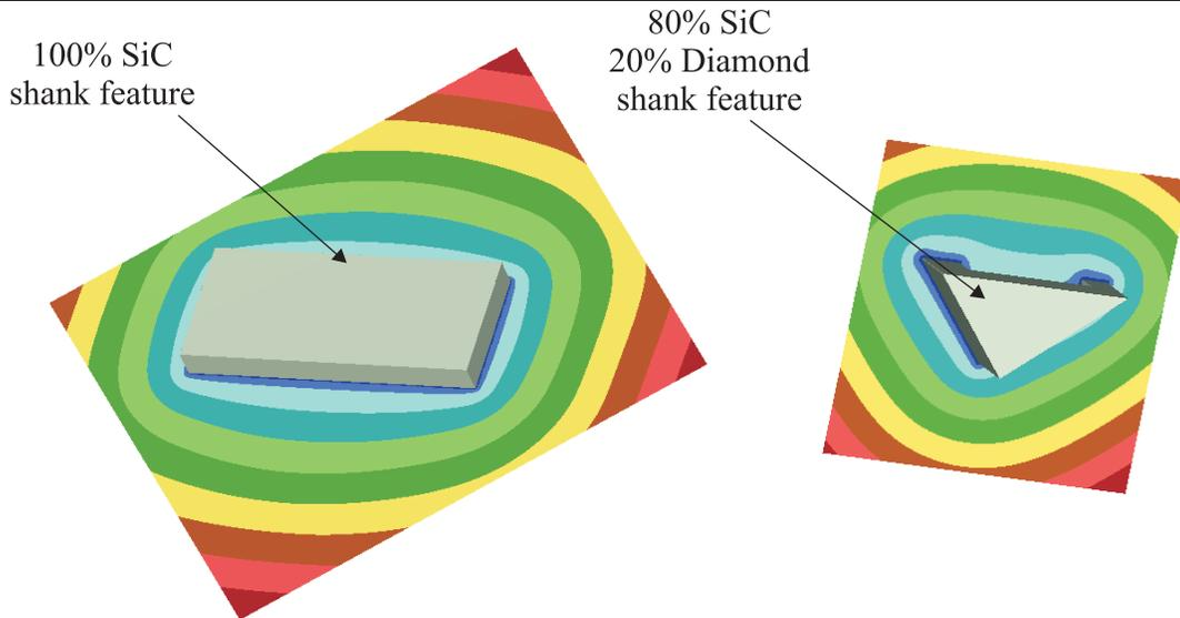
Figure 3: Approximate distance fields for two material features of the diamond cutter tool of Figure 1, are normalized to the second order, and the distance fields are shown on the midsection.
