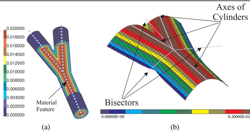
Figure 8: Refractive index distribution of a radial GRIN Y-branching waveguide for optical communications. (a) Distribution  $(0.02 - 50u^2)$  is specified explicitly for the Y-shaped one-dimensional skeleton. (b) Magnified distribution plotted as a surface over a 2D section: analytic everywhere away from the feature, including the points on bisectors where the exact distance field would not be differentiable.
