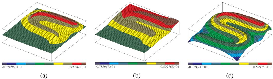
Figure 7: Non-constant material function on a feature with derivative control: (a) material function  $F_0 = ye^{-1.5u}$  is prescribed on the S-shaped feature; (b) conditioned function  $F_0^*$  agrees with  $F^0$  on the feature but behaves as a constant function in the direction normal to the S-curve; (c) first derivative in the canonical form of the material function,  $F_1 = -4$ , is specified on all points of the curve in addition to its value  $F_0$ .
