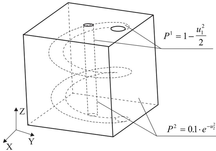
Figure 13: Three-dimensional material modeling problem requires constructing a material function for the solid from the material functions associated with the two features as shown.
