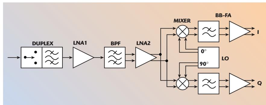
▲ Fig. 6 Direct-conversion receiver including filter.
