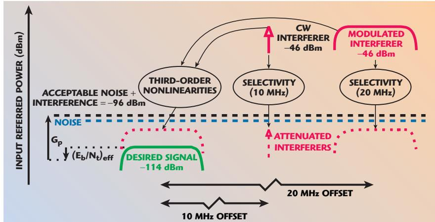
▲ Fig. 4 Intermodulation test.
