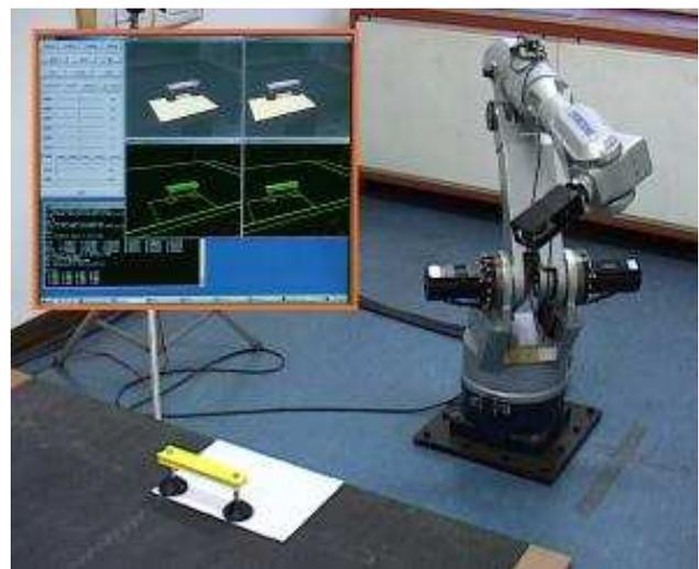
Figure 3: Hardware setup and man-machine interface for pose registration tests with a camera on the robot wrist.
