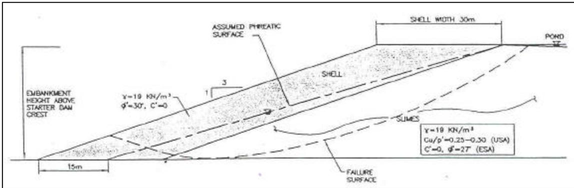
Figure 5. Stability analysis section.
