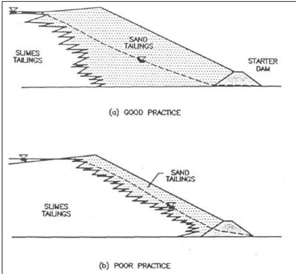
Figure 1. Idealized sections of upstream tailings dams.
