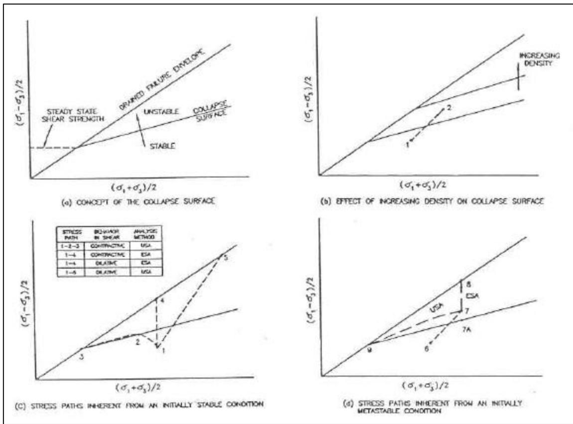
Figure 2. Collapse surface framework for comparison of USA and ESA approaches.
