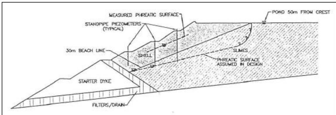
Figure 4. Typical design section of upstream dams reviewed.
