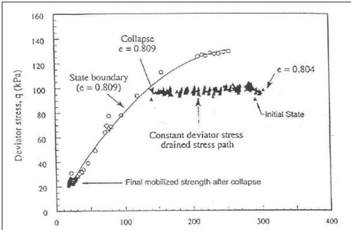
Figure 3. State boundary defined by void ratio 0/809 and constant deviator ( $q=100\text{kPa}$ ) drained stress path. After Sasitharan et al (1993).
