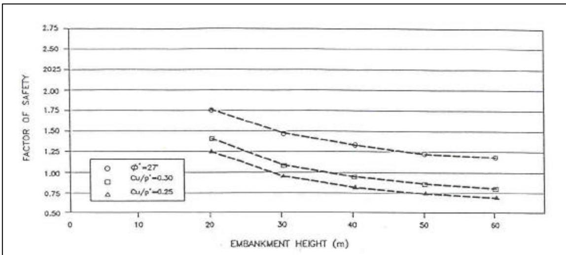
Figure 6. Results of preliminary stability analyses.
