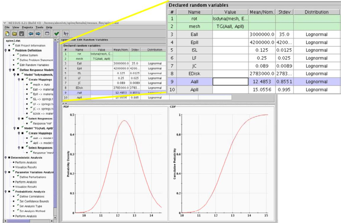
Figure 2. NESSUS<sup>®</sup> allows for random variables to be defined with a mean, standard deviation and distribution type.
