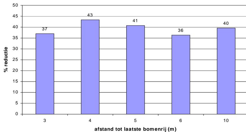
**Figure 10.** Mean drift reduction (session 1-3) at different distances from the last tree row when spraying the outward three rows and the last row only from the outside in a nearly bare tree situation (after Wenneker *et al.*, 2001b)
