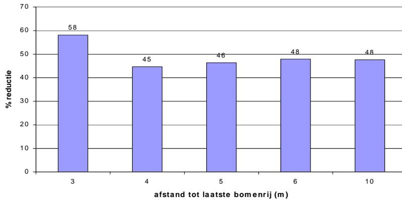
**Figure 9.** Mean drift reduction (session 1-3) at different distances from the last tree row when spraying the outward three rows and the last row only from the outside in a full developed canopy situation (after Wenneker *et al.*, 2001b)
