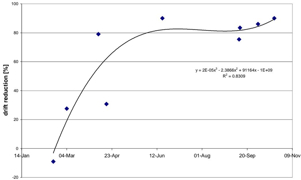
**Figure 7** Spray drift reduction of an alder windbreak at different dates during the growing season when spraying an apple orchard (based on data of Porskamp *et al.*, 1994; Wenneker *et al.*, 2004a)
