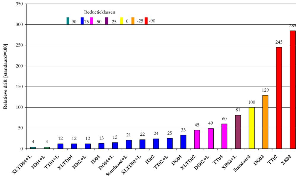
**Figure 3. Relative spray drift deposition on 2-3 m distance from the last nozzle for different nozzles and nozzles in combination with air assistance (+A) when spraying potatoes with a spray volume of 300 l/ha (04 nozzles) and 150 l/ha (02 nozzles). Standard nozzle is XR 110.04 (=100)**
