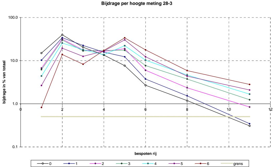
**Figure 6** Contribution of individual row sprayings (1-11) to airborne spray drift on 5m distance from the last tree row in an apple orchard averaged for different heights (0-6m)
