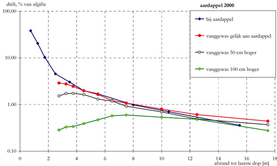
**Figure 5. Spray drift when spraying a potato crop (2000) with a windbreak crop of different heights next to it (equal height as the potato crop, +50 and +100 cm higher than potato crop canopy), without air assistance (after: Michielsen et al., 2003)**
