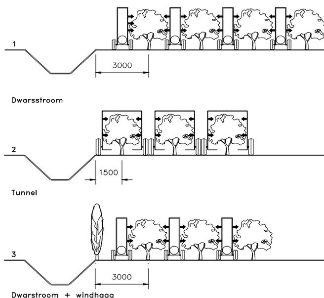
**Figure 2. Representation of used spraying systems and situations in orchard spraying.**
