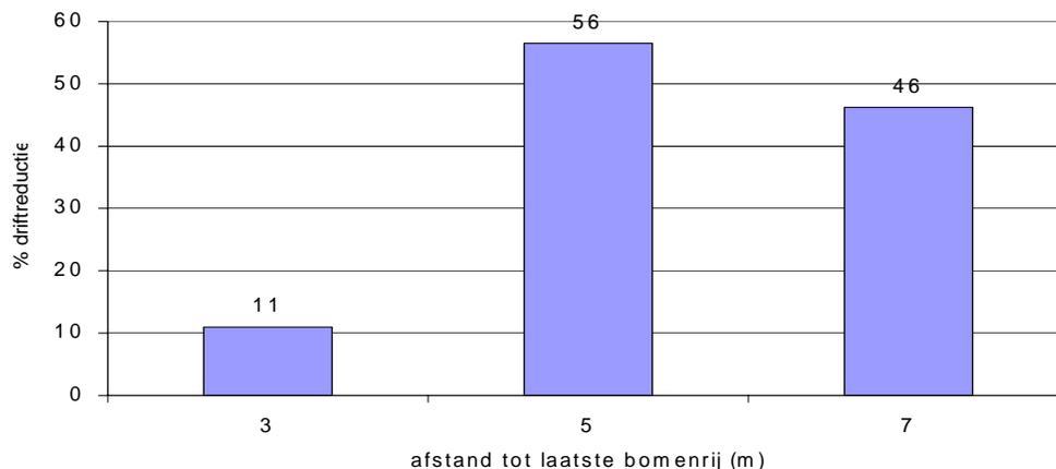
**Figure 11: Mean drift reduction of a reed vegetation in the ditch at different distances from the last tree row when spraying the outward 2 rows of trees with a cross-flow sprayer (full-leaf situation) (Van de Zande et al., 2001)**
