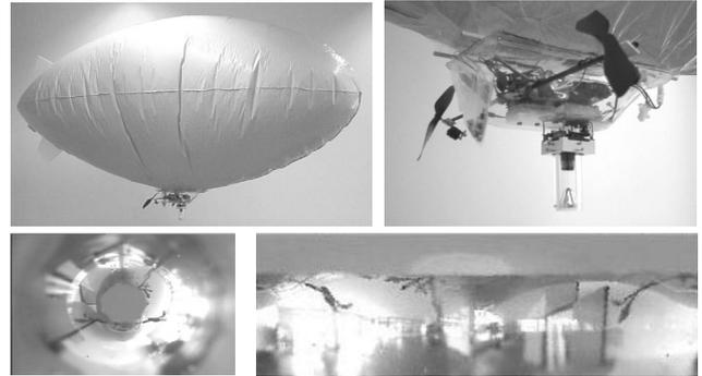
**Figure 2. Top:** The autonomous flying robot, *Melissa*, and its gondola. **Bottom:** An image obtained by the panoramic vision system and its log-polar transformed image, which is also used in the experiments.
