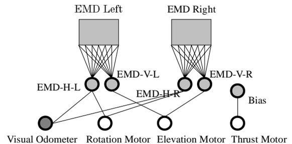
**Figure 3.** The sensory-motor control circuit.
