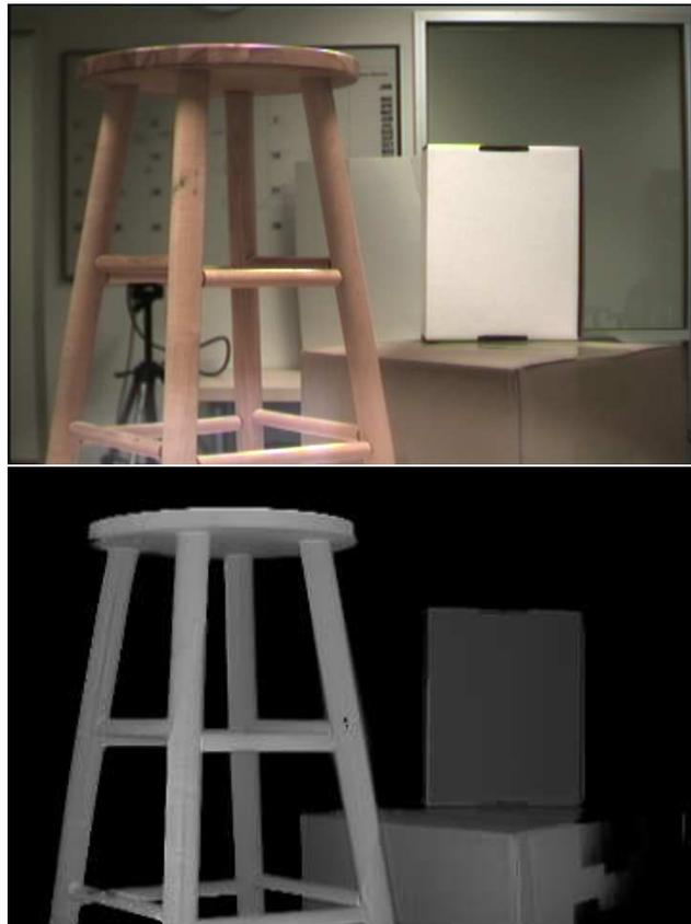
Figure 2: An example of a depth image produced by an SLP sensor. Far objects are shaded with increasingly darker tones of grey.
