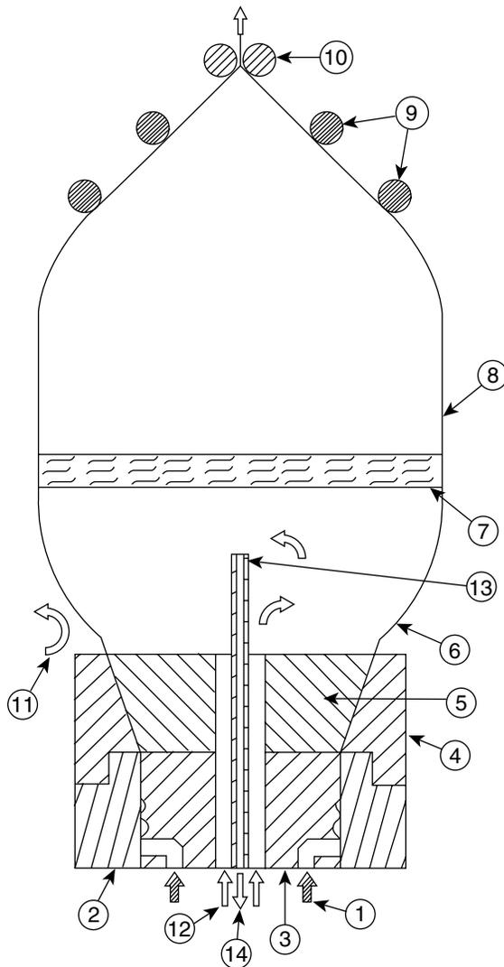
**Fig. 3** Schematic of spiral mandrel blown film die operation: (1) ring-shaped melt distribution; (2) die body; (3) spiral flow mandrel; (4) sizing ring; (5) spreader; (6) film bubble; (7) frost line; (8) solidified film; (9) bubble collapsing rollers; (10) nip rollers; (11) external bubble cooling air; (12) internal bubble cooling air inlet; (13) internal bubble cooling pipe; and (14) heated internal bubble air return.
