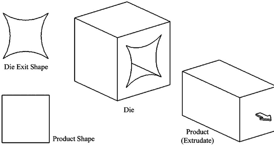
Fig. 5 Irregular die shapes required for regular extrudates.
