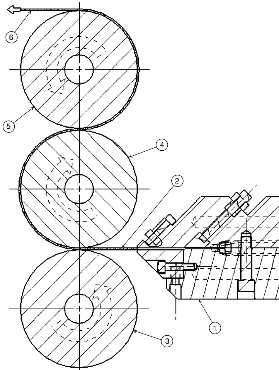
**Fig. 9** Chill roll stack for sheet extrusion: (1) sheet die with flow restrictor; (2) molten sheet extrudate; (3) lower chill roll (all chill rolls temperature controlled); (4) middle chill roll (imparts gloss/surface texture to sheet); (5) upper chill roll; and (6) solidified sheet.
