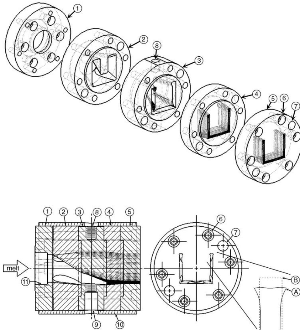
**Fig. 7** U-Profile stack die: exploded view (top); section view (lower left); and end view (lower right): (1) extruder mounting plate; (2) die adapter plate; (3) transition plate; (4) preland plate; (5) die land plate; (6) die bolt hole; (7) alignment dowel pin hole; (8) thermocouple well; (9) pressure transducer port; (10) heater band; (11) breaker plate recess. Detail (lower right): (A) die exit profile and (B) product profile.
