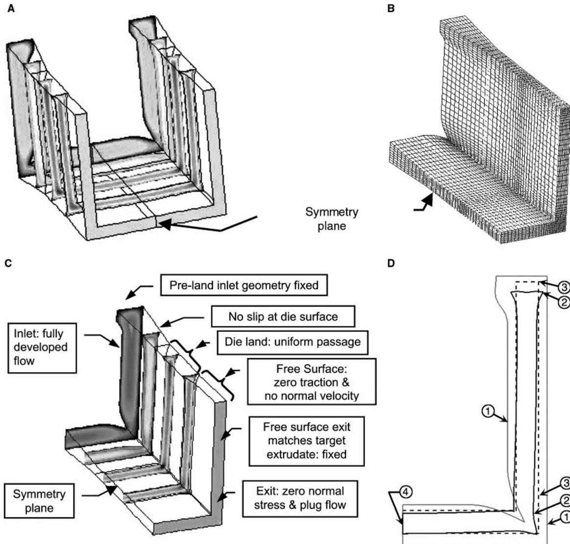
**Fig. 13** Computational model for U-Profile die design: (A) preland, die land, and free surface as computational domain; (B) finite element mesh (symmetry exploited to reduce computational requirements); (C) boundary conditions for simulation of polymer flow through die and extrudate free surface; and (D) relevant profiles: (1) preland inlet; (2) die land (uniform along flow length); (3) final free surface (target extrudate profile); and (4) symmetry plane.
