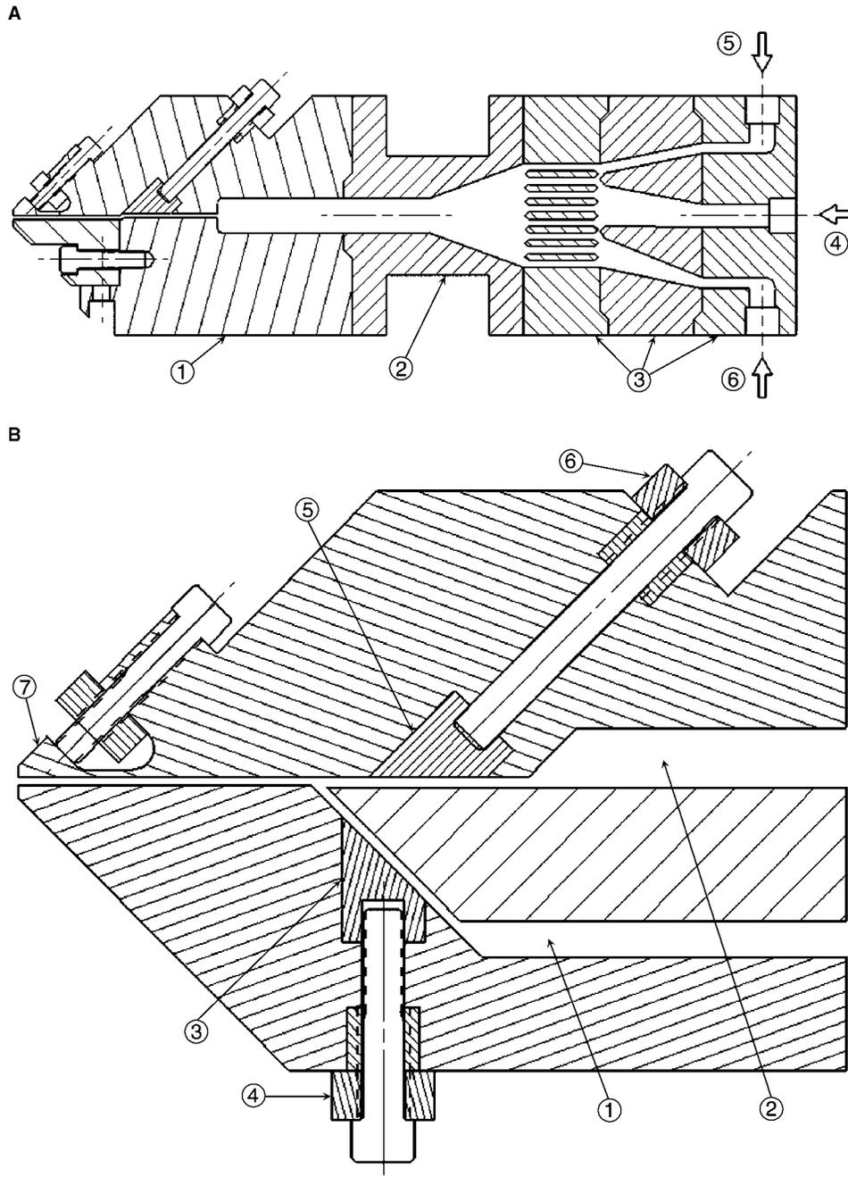
**Fig. 8** Coextrusion feed block manifold and sheet die (A): (1) sheet die with flow restriction; (2) adapter plate; (3) feed block assembly; (4) core material layer inlet; (5) upper material layer inlet; (6) lower material layer inlet; and coextrusion multimanifold sheet die (B): (1) lower melt channel; (2) upper melt channel; (3) lower choker bar; (4) lower choker bar adjustment bolt; (5) upper choker bar; (6) upper choker bar adjustment bolt; (7) flex lip.
