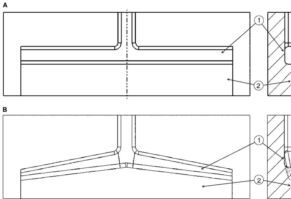
**Fig. 2** Comparing designs of T-type die (A) [(1) constant cross-section manifold; (2) constant land length] to coat hanger-type die (B) [(1) manifold cross-section decreases as distance from centerline increases; (2) land length becomes shorter farther from the centerline of the die].
