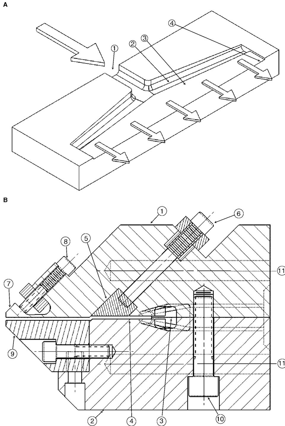
**Fig. 1** Coat hanger-type sheet die concept (A): (1) central inlet port; (2) manifold (distributes melt); (3) island (along with manifold, provides uniform pressure drop from inlet to die lip); (4) die lip (die exit forms a wide slit); and schematic of sheet die (B): (1) upper die plate; (2) lower die plate; (3) manifold; (4) island; (5) choker bar; (6) choker bar adjustment bolt; (7) flex die lip; (8) flex lip adjustment bolt; (9) lower lip; (10) die bolt; (11) heater cartridge.
