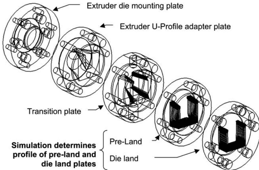
Fig. 12 U-Profile die plates designed with CFD simulation.
