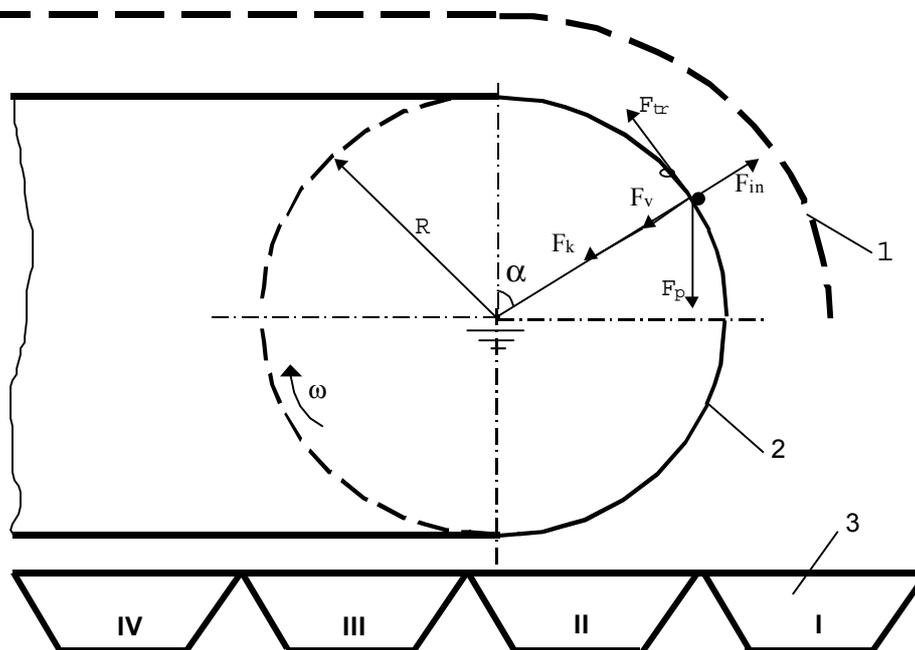
Figure 1. The scheme of transporter type electric separator: 1-potential electrode; 2- grounded electrode; 3-classifier pans
