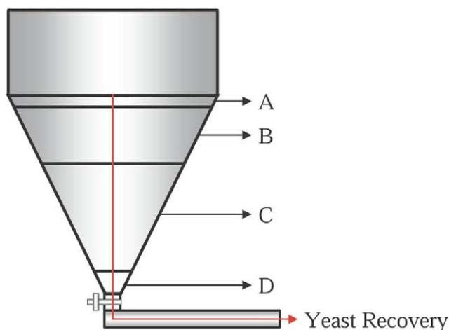
Fig. 1. Schematic illustration of the stratification of yeast during sedimentation. (A) indicates the youngest cell fraction, (D) the predominantly aged fraction. (A), (B) and (C) represent the fractions reused for successive fermentations with traditional cropping techniques. Fraction (C) represents yeast removed from the vessel during warm cropping.
