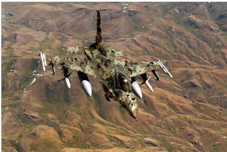
Figure 5. Camouflage can be dynamic in several ways, including simple movement. A Jordanian F-16 painted in HyperStealth Biotechnology Corp.'s fractal-like camouflage.
