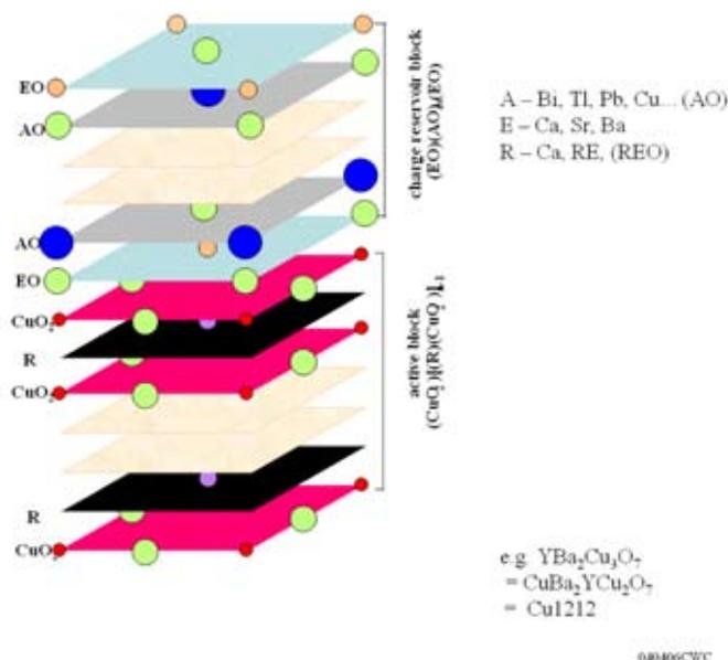
Fig. 4: The layered structure of HTS cuprates.
