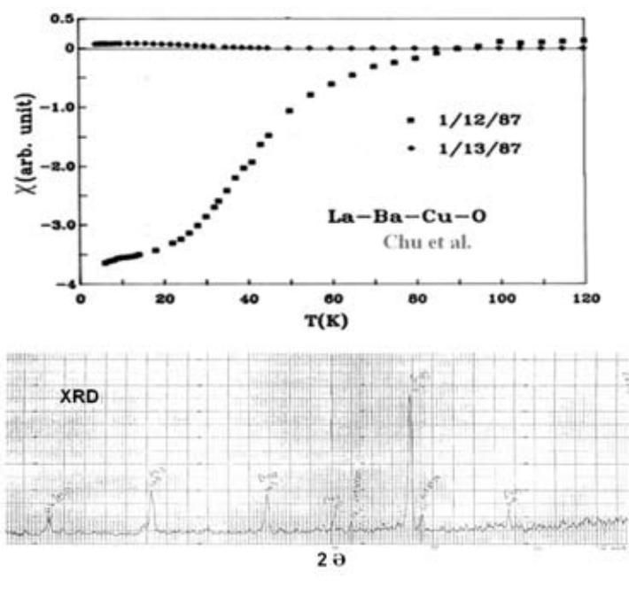
Fig. 2: The first definitive sign of superconductivity above 77 K.
