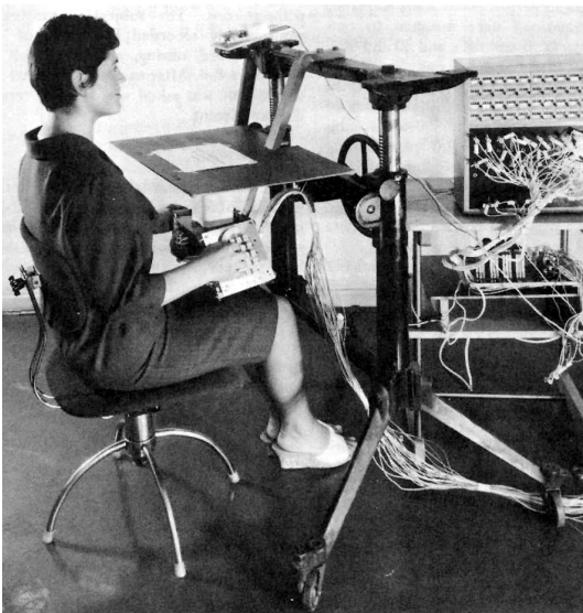
Figure 4. Experimental setup for the Kroemer studies. Note that the participant cannot see the keyboard during the typing task (Kroemer, 1972).
