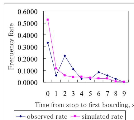
Figure 10. Comparison of observed and simulated dwell time component (Duration from instant of stopping to time of boarding of first passenger)
