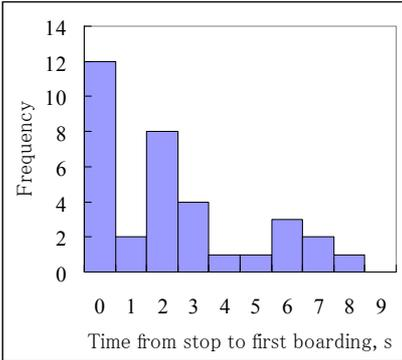
Figure 3. Frequency distribution of dwell time component (Duration from instant of stopping to time of boarding of first passenger)
