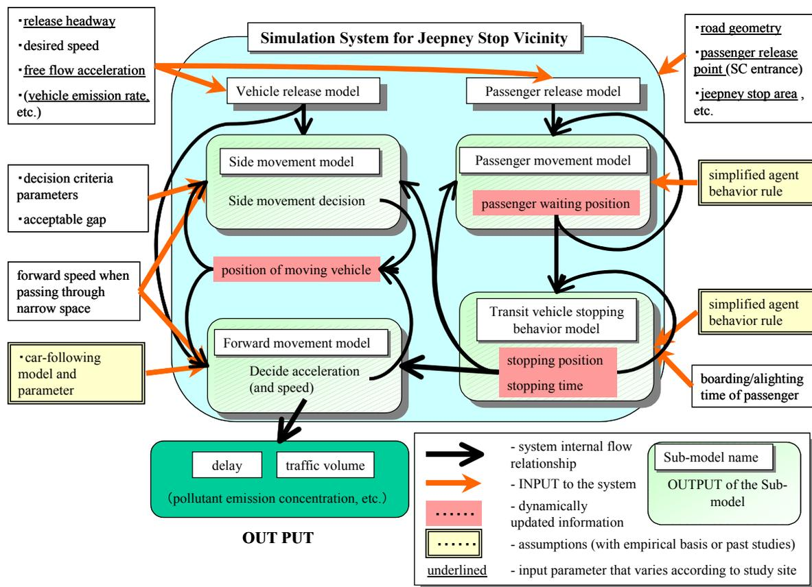
Figure 7. Structure of the simulation model system
