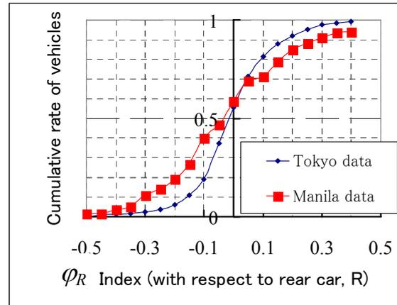
Figures 1 (left) & 2 (right). Cumulative rate of vehicles for varying values of  $\varphi$ . (Index  $\varphi$  is rate of change of distance headway, a measure of lane changing aggressiveness; Tokyo data from Nakamura *et al.*, 1992)
