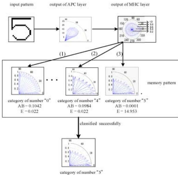
Fig. 9 Classification of standard pattern of number "5".
