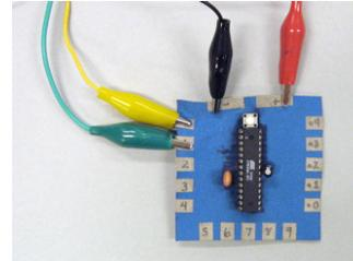
**Figure 5. Alligator clips are used to connect microcontroller modules to other devices.**
