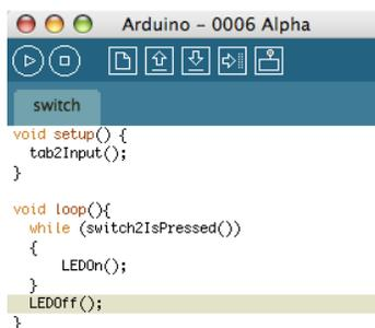
Figure 2. The Arduino IDE.
