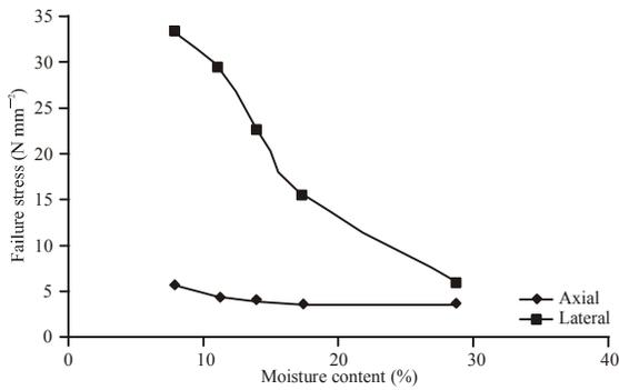
Fig. 3: Failure stress at seedcoat rupture as a function of moisture content
