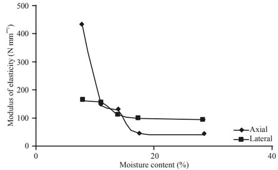
Fig. 4: Modulus of elasticity at seedcoat as a function of moisture content
