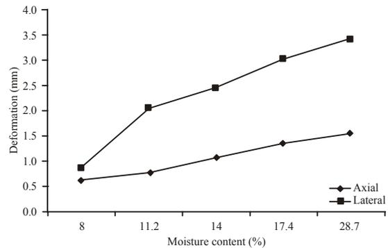
Fig. 5: Deformation at seedcoat rupture as a function of moisture content
