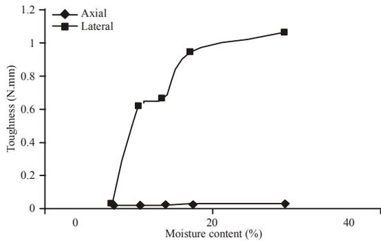
Fig. 2: Toughness at seedcoat rupture as a function of moisture content
