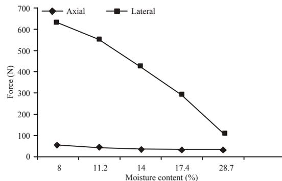
Fig. 1: Force to cause seedcoat rupture as a function of moisture content
