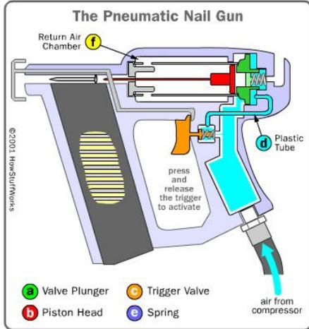
Figure 1: A schematic showing the mechanics of the nail gun.
