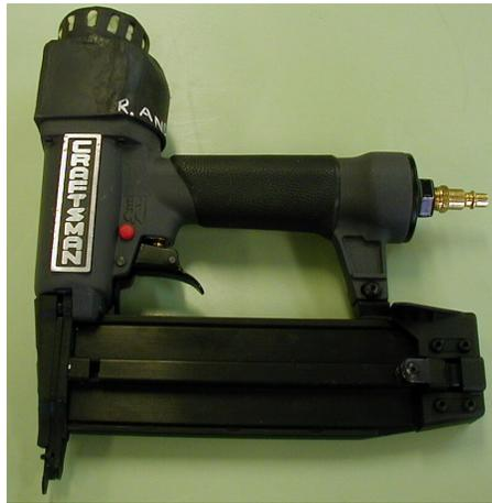
Figure 7: Nail gun with muffler.
