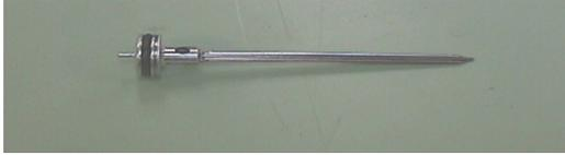
Figure 5: Original piston assembly.
