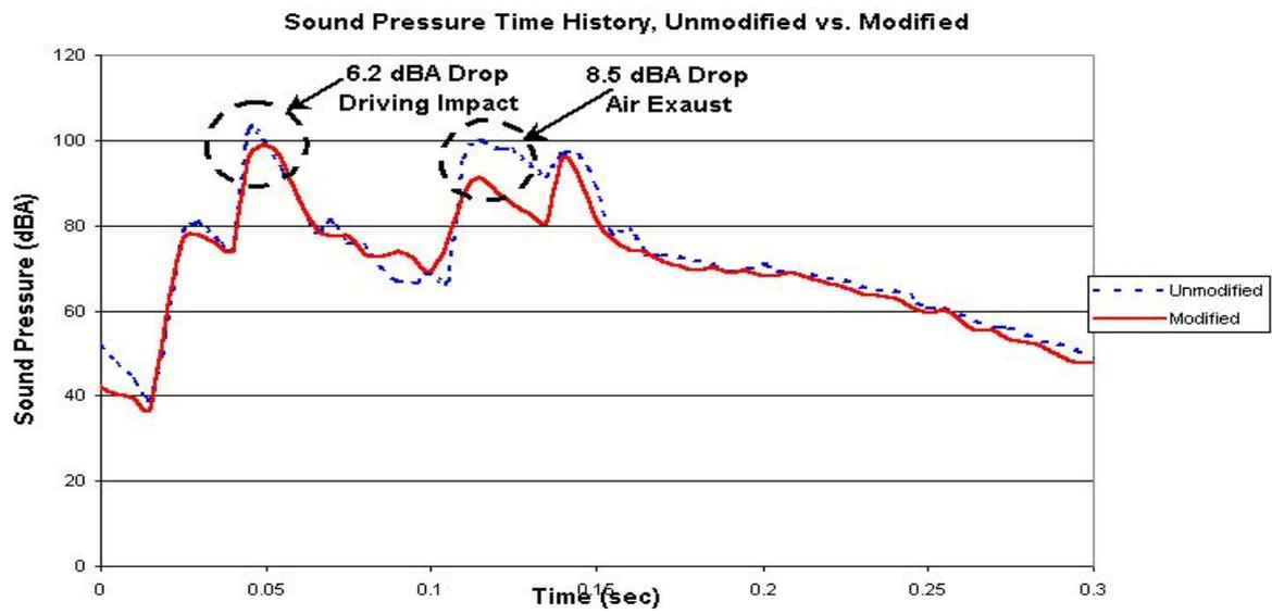
Figure 8: Sound pressure levels, unmodified vs. modified.
