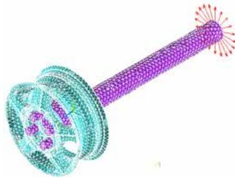
Figure 2. Simulating the dynamic cornering fatigue test
