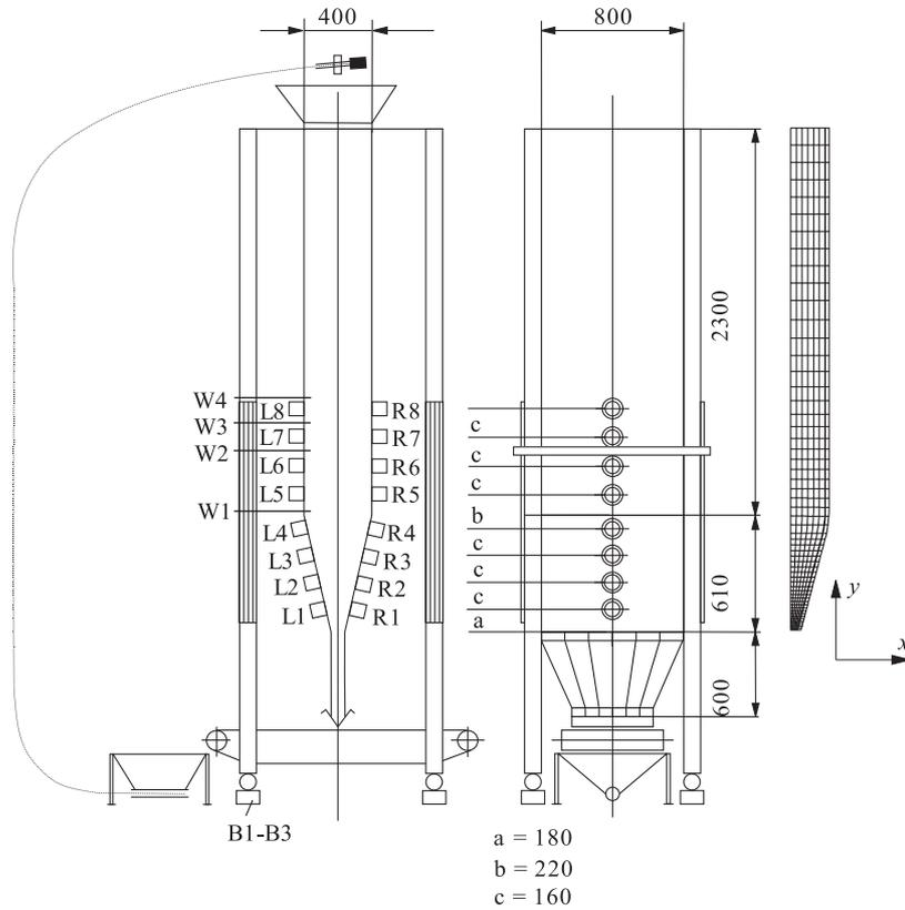
**Figure 1.** Experimental setup and FE grid: positions of load cells and strain gauges for the measurement of the stresses, wall deformations and silo mass; the FE grid represents a symmetric part of the silo
