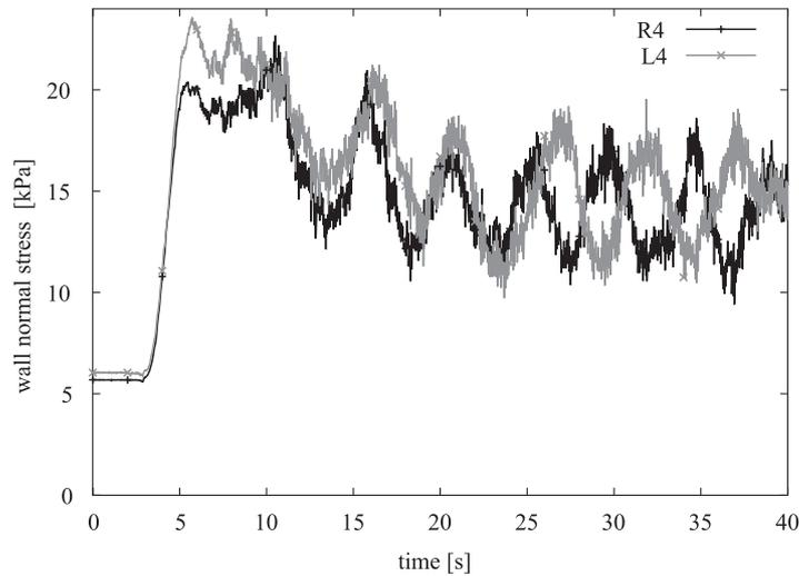
**Figure 8.** Measured stress distribution: alternating stress fluctuation in the hopper
