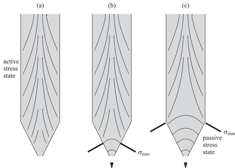
**Figure 4.** Principle stress trajectories and maximum normal wall stress: change from the active to the passive stress state in the hopper and upward movement of the stress peak at the beginning of discharge
