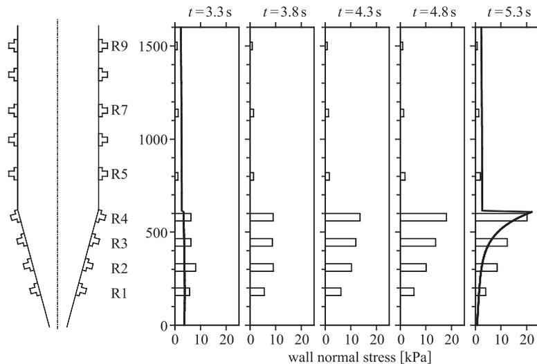
**Figure 5.** Wall normal stress in the experimental silo at various time steps: measured results at load cell positions R (bars) and analytical results of the filling state and the discharge state (lines) [21]
