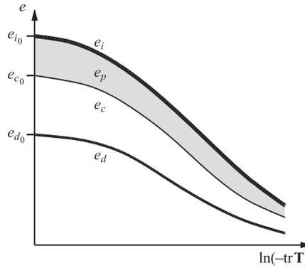
**Figure 2.** Void ratio, dependence on volumetric (hydrostatic) stress;  $e_i$  – upper limit,  $e_d$  – lower limit,  $e_c$  – critical void ratio and  $e_p$  – the SOM region (swept out of memory)
